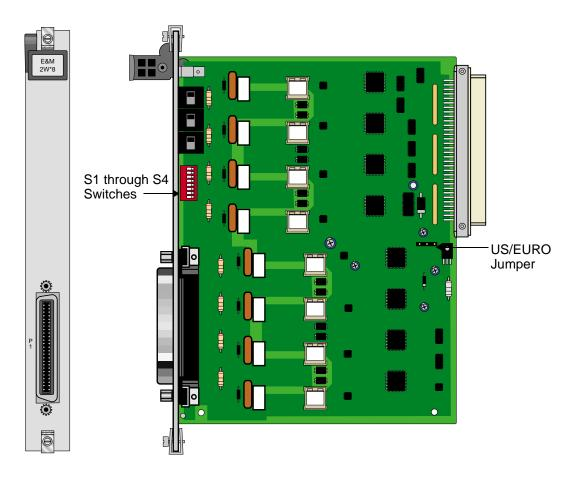
Figure 1-1.Typical E&M Card Switches
