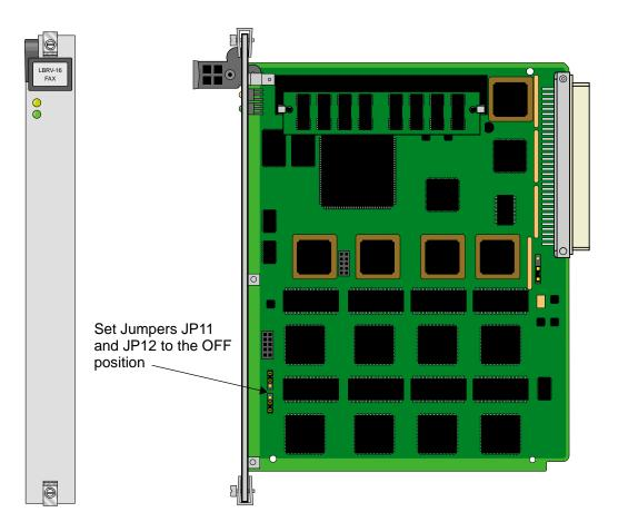
Figure 7-3.LBRV-16 FAX Card Jumper Settings
