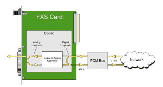
Figure 2-3.FXS Card Loopbacks
