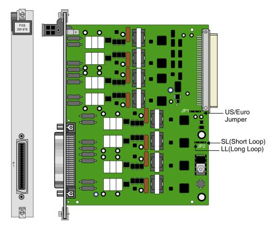
Figure 2-1.FXS 2W\*8-6 Card Jumpers Settings
