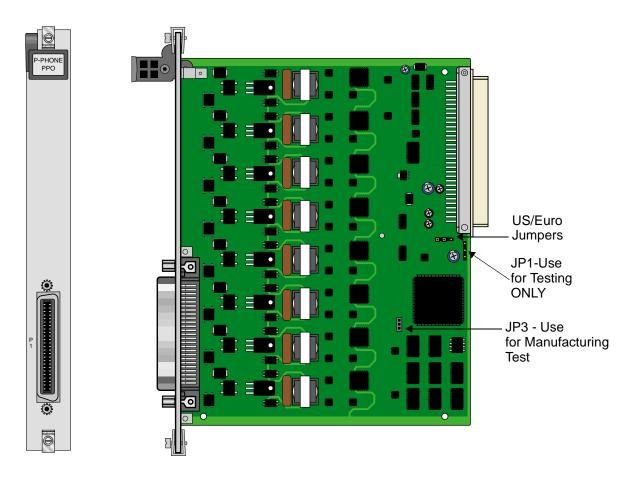
Figure 8-1.P-Phone PPO and PPS Cards Jumper Settings
