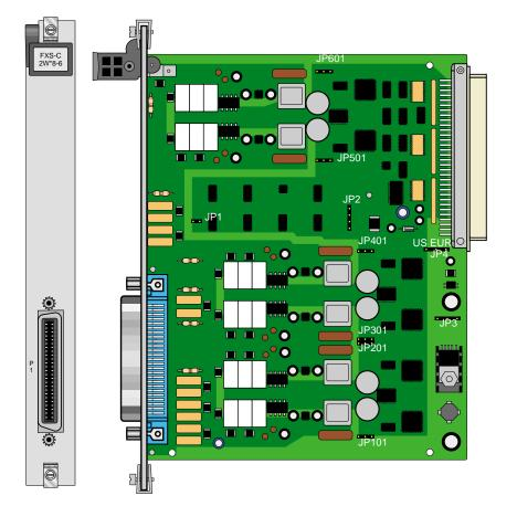
Figure 5-1.Jumper Settings for FXS Coin Card
