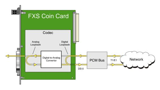
Figure 5-3.FXS Coin Card Loopbacks
