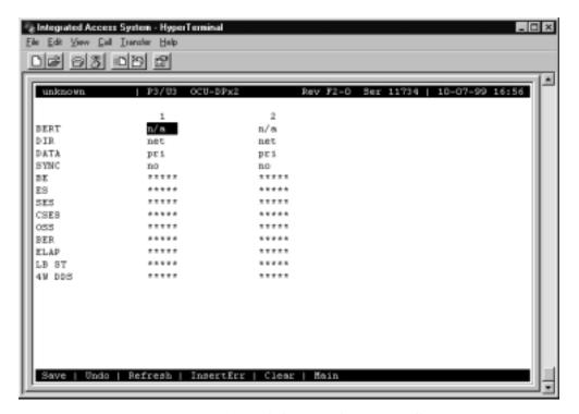
Figure 4-10. Typical OCU-DP Card Test Screen
