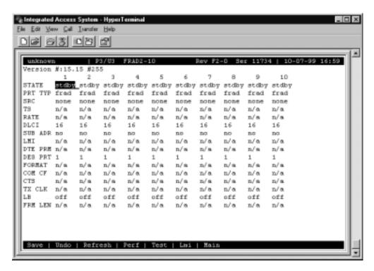
Figure 5-2. Typical FRAD Card Main Screen
