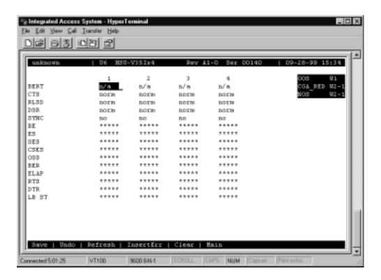
Figure 1-15. Typical HSU Card Test Screen
