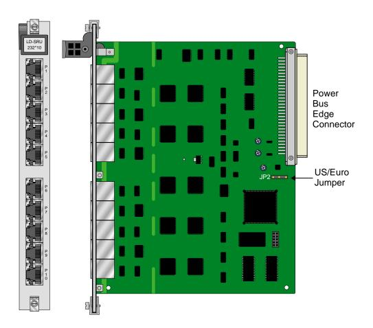
Figure 3-4.SRU-LD\*10 Card Jumper Settings
