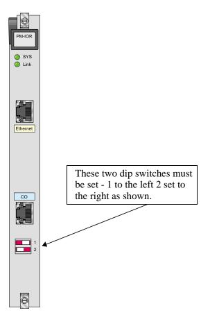
Figure 9-1.PM-IOR Card Dip-switch settings (828060)
