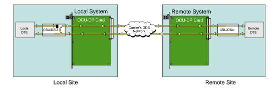
Figure 4-8.OCU Remote Loopback (csu-u option)
