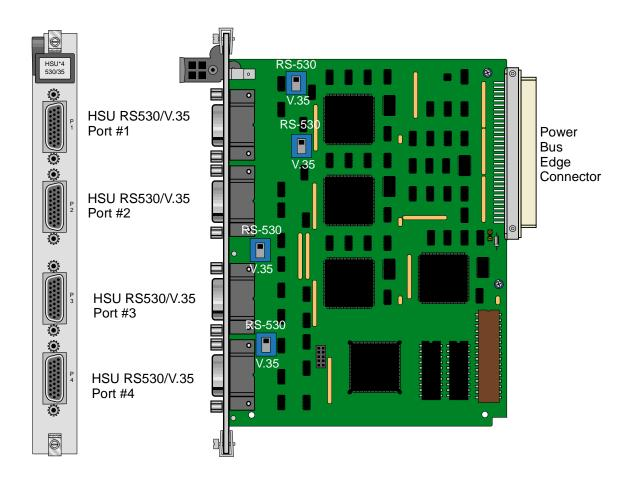
Figure 1-4.Four-Port HSU 530/35 Card Switches
