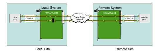
Figure 5-3.DTE Loopback
