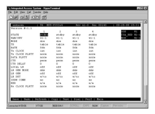
Figure 1-8. Typical HSU Card Main Screen
