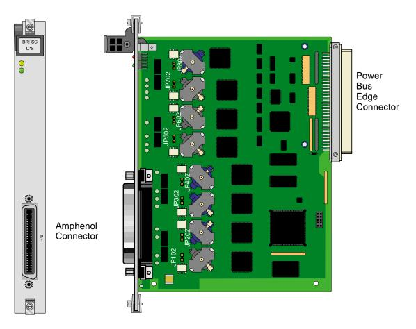
Figure 8-3.BRI-SC U\*8 Card Sealing Current Jumpers
