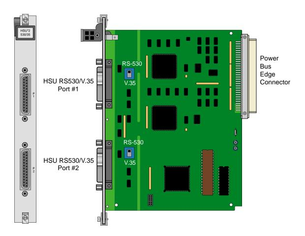
Figure 1-1.Two-Port HSU 530/35 Card Switches
