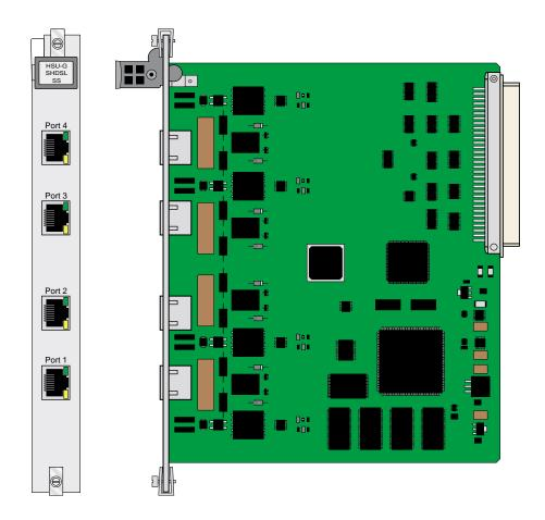
Figure 10-1. Four-Port SHDSL Card ()
