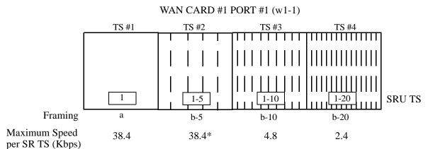
\*Speeds greater than 9.6Kbps will occupy contiguous SRU Timeslots in 9.6Kbps increments (i.e. a 19.2Kbps circuit would take SRU timeslots #1 and #2)
