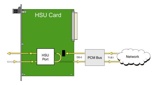
Figure 1-10.Local DTE Loopback
