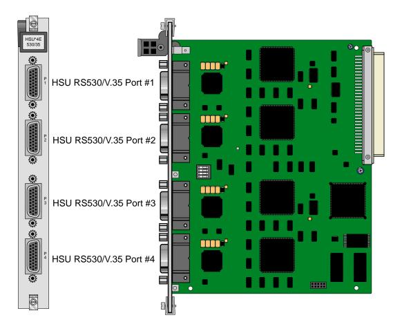
Figure 1-5.Four-Port HSU\*4E 530/35 SS Card Switches
