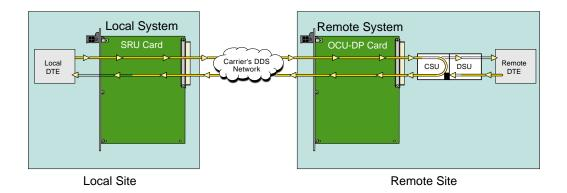
Figure 3-9.Inband Remote CSU Loopback
