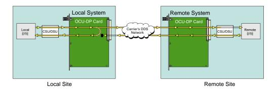
Figure 4-3.OCU Local Loopback (dte option)
