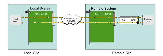
Figure 1-14.Remote DSU Loopback
