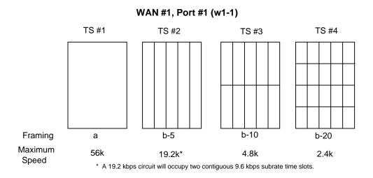
Figure 4-2.Data Frames, Rates, and Time Slot Assignments
