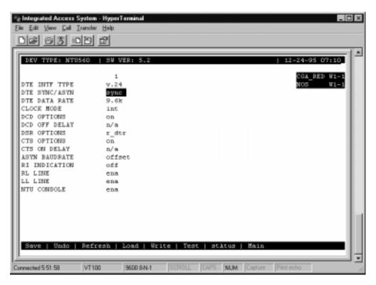
Figure 8-14.Remote NTU Configuration Screen (2560/2561 or 2200E/2201E)
