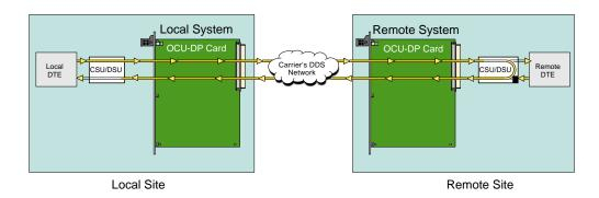
Figure 4-7.OCU Remote Loopback (csu-n option)
