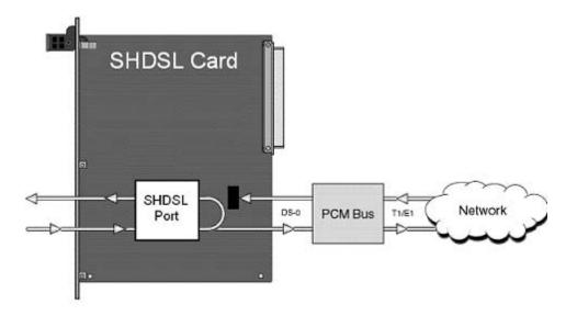
Figure 10-4. Local DTE Loopback
