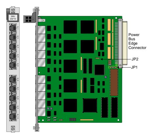
Figure 3-2.SRU 232\*10 C&D Bus Jumper Settings
