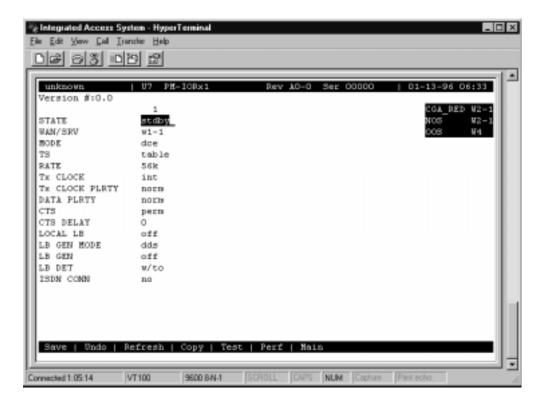
Figure 9-2. Typical PM-IOR Card Main Screen
