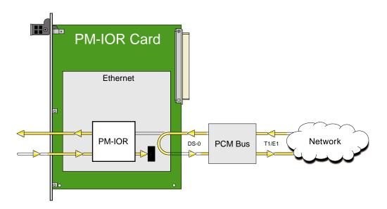
Figure 9-4.Local DTE Loopback
