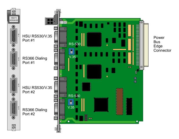
Figure 1-2.HSU-AD 530/35 Card Switches
