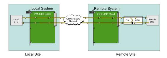
Figure 9-8.Remote DSU Loopback
