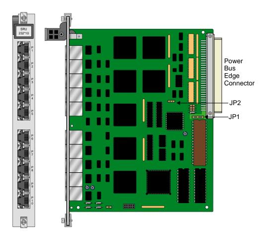
Figure 3-1.SRU 232\*10 Jumper Settings
