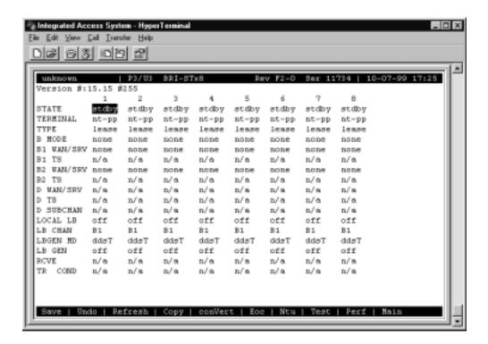
Figure 8-7. Typical BRI-ST\*8 Card Main Screen
