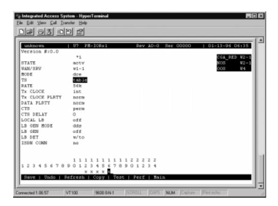
Figure 9-3. Typical PM-IOR Port time slot Assignment Screen
