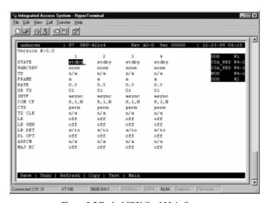
Figure 3-5. Typical SRU Card Main Screen
