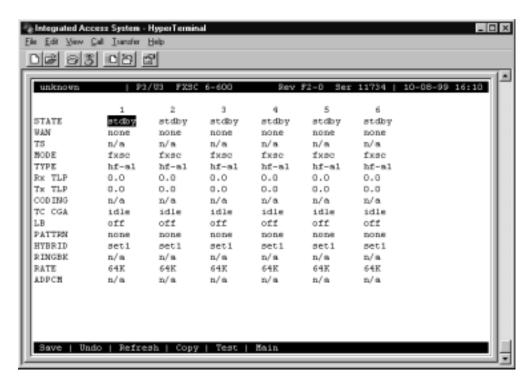
Figure 5-2. Typical FXS Coin Card Main Screen
