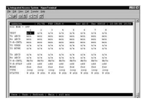
Figure 2-4. Typical FXS Card Test Screen
