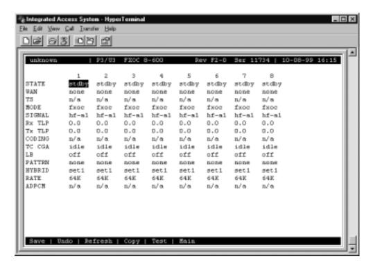
Figure 6-2. Typical FXO Coin Card Main Screen
