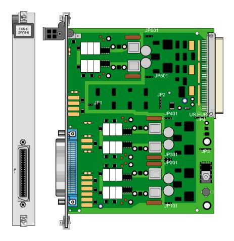
Figure 5-1. Jumper Settings for FXS Coin Card
