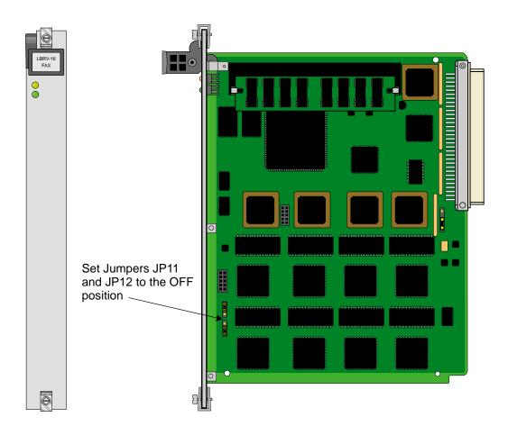
Figure 7-3.LBRV-16 FAX Card Jumper Settings
