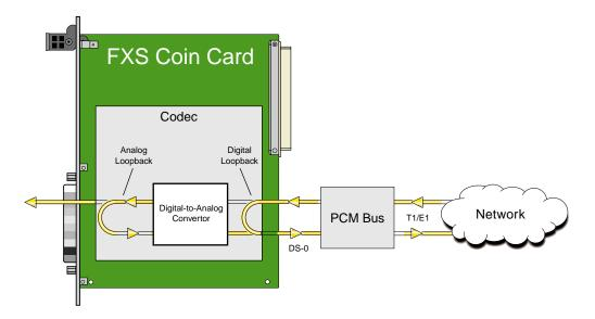
Figure 5-3.FXS Coin Card Loopbacks
