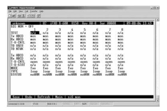
Figure 4-4. Typical iFXO Card Test Screen
