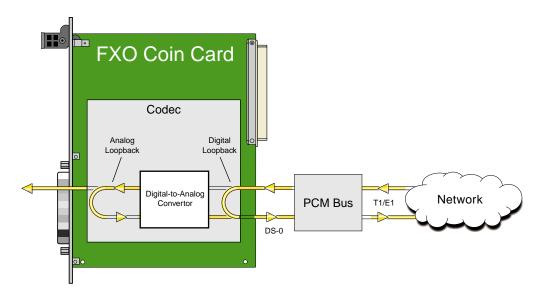
Figure 6-3.FXO Coin Card Loopbacks
