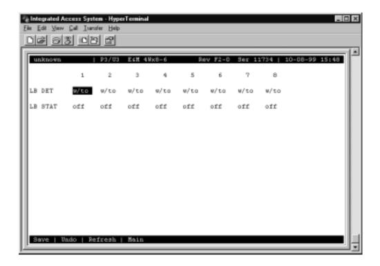
Figure 1-6. Typical E&M Loopback Screen
