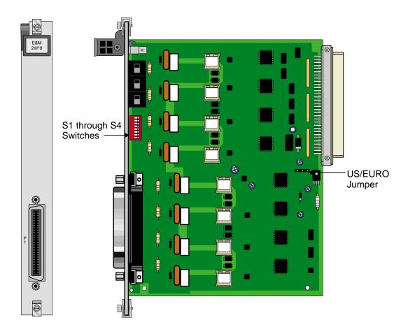
Figure 1-1. Typical E&M Card Switches
