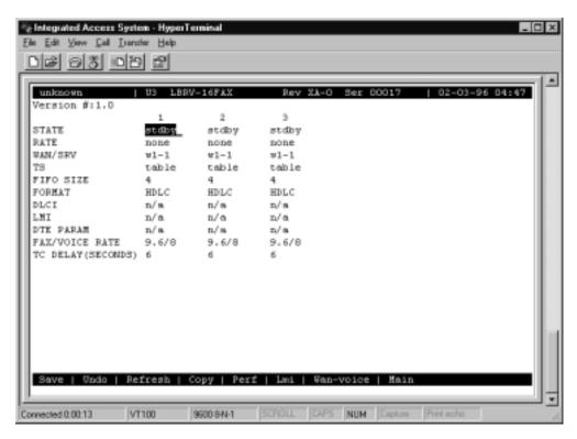
Figure 7-4.LBRV-16 FAX Card Main Configuration Screen
