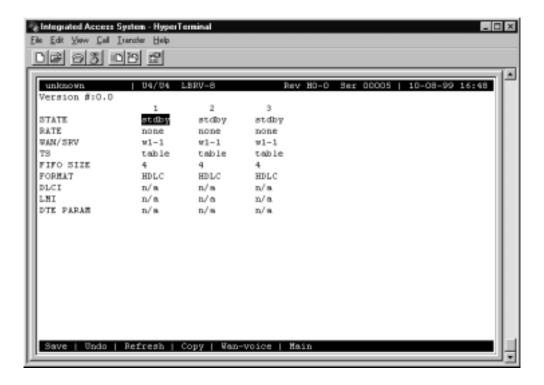
Figure 7-1.LBRV-8 FAX Card Main Configuration Screen
