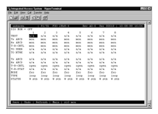
Figure 3-4. Typical FXO Card Test Screen
