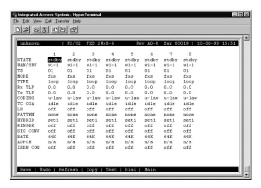
Figure 2-2. Typical FXS Card Main Screen
