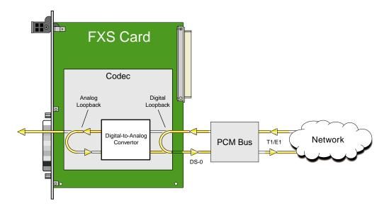
Figure 2-3. FXS Card Loopbacks
