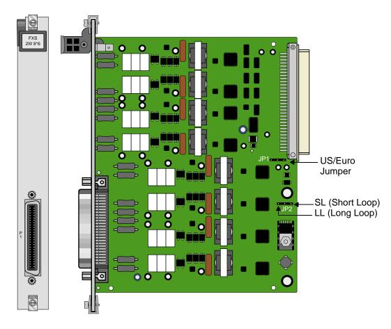
Figure 2-1. FXS 2W\*8-6 Card Jumpers Settings
