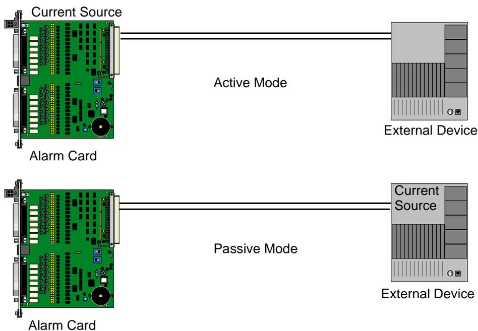
**Figure 1-4. Active and Passive Alarm Sensor Modes**
