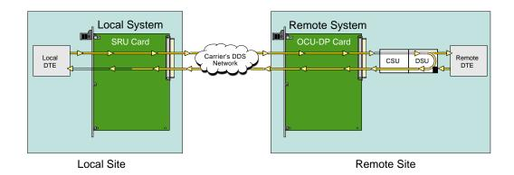
Figure 3-10. Inband Remote DSU Loopback
