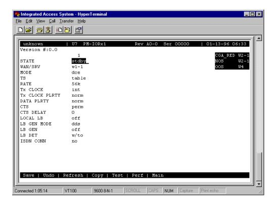
Figure 9-2. Typical PM-IOR Card Main Screen
