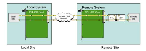
Figure 9-7. Remote CSU Loopback
