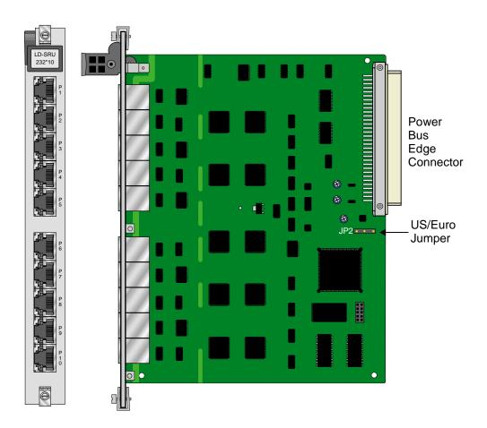
Figure 3-4. SRU-LD\*10 Card Jumper Settings
