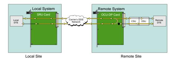
Figure 3-8. Inband Remote SRU Loopback
