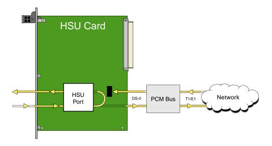
Figure 1-10. Local DTE Loopback
