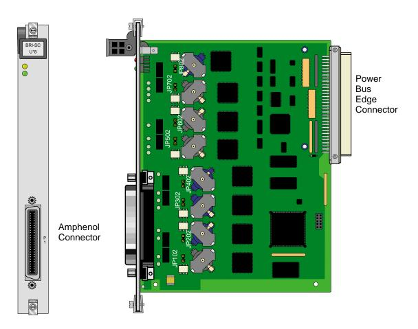
Figure 8-3. BRI-SC U\*8 Card Sealing Current Jumpers
