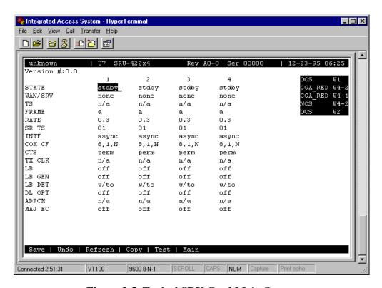
Figure 3-5. Typical SRU Card Main Screen
