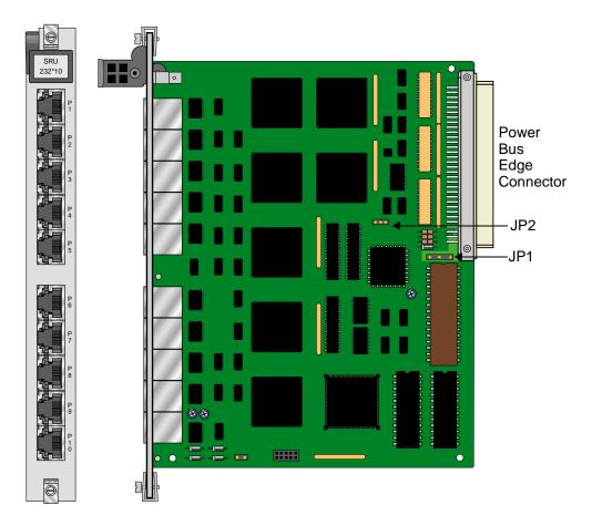
Figure 3-1. SRU 232\*10 Jumper Settings
