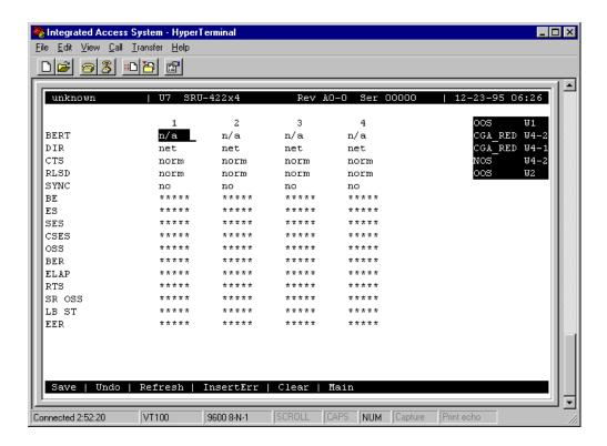
Figure 3-12. Typical SRU Card Test Screen
