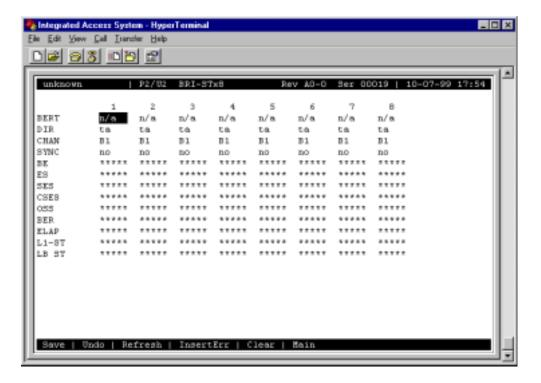
Figure 8-19. Typical BRI-ST\*8 Card Test Screen
