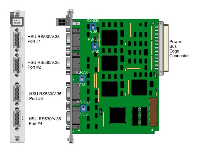
Figure 1-4. Four-Port HSU 530/35 Card Switches
