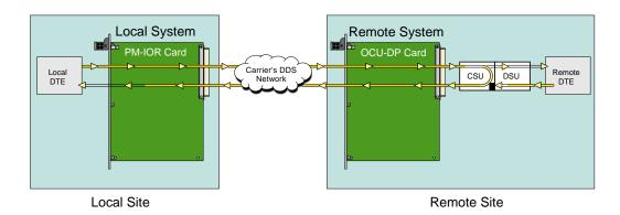
Figure 9-8. Remote DSU Loopback
