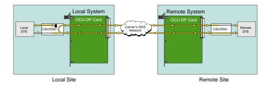
Figure 4-8. OCU Remote Loopback (csu-u option)
