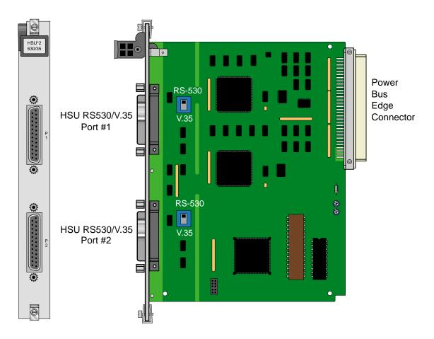
Figure 1-1. Two-Port HSU 530/35 Card Switches
