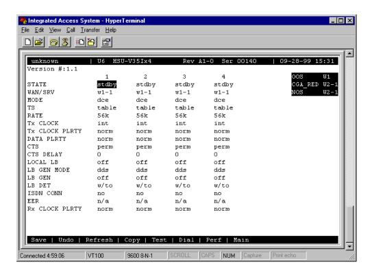
Figure 1-8. Typical HSU Card Main Screen
