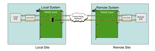
Figure 5-3. DTE Loopback
