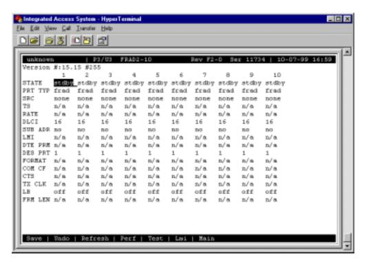
Figure 5-2. Typical FRAD Card Main Screen
