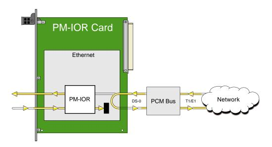
Figure 9-4. Local DTE Loopback
