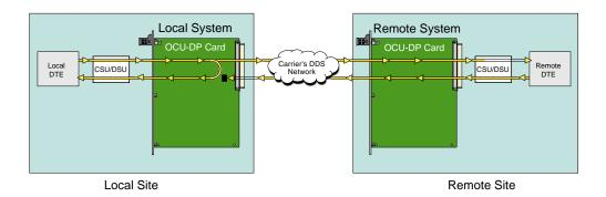
Figure 4-3. OCU Local Loopback (dte option)
