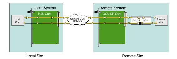
Figure 1-13. Remote CSU Loopback
