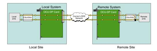
Figure 4-7. OCU Remote Loopback (csu-n option)
