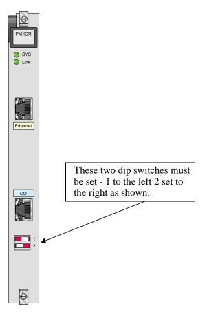
Figure 9-1. PM-IOR Card Dip-switch settings (828060)
