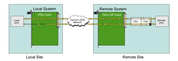
Figure 1-14. Remote DSU Loopback
