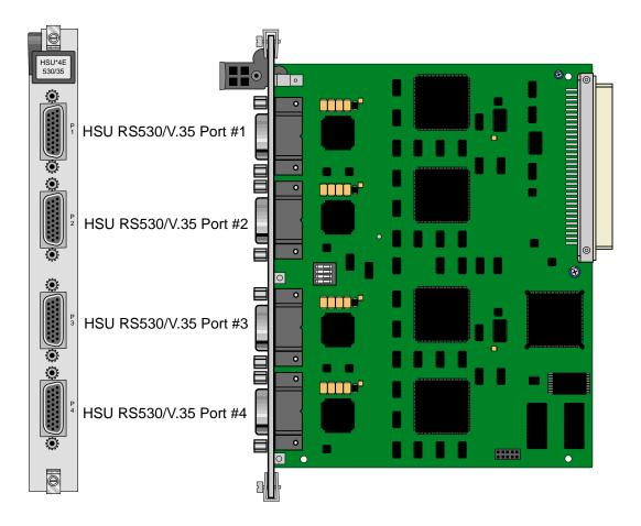
Figure 1-5. Four-Port HSU\*4E 530/35 SS Card Switches
