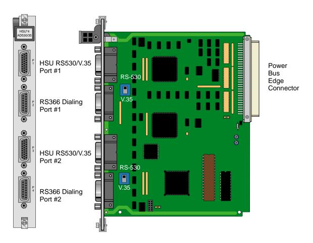
Figure 1-2. HSU-AD 530/35 Card Switches
