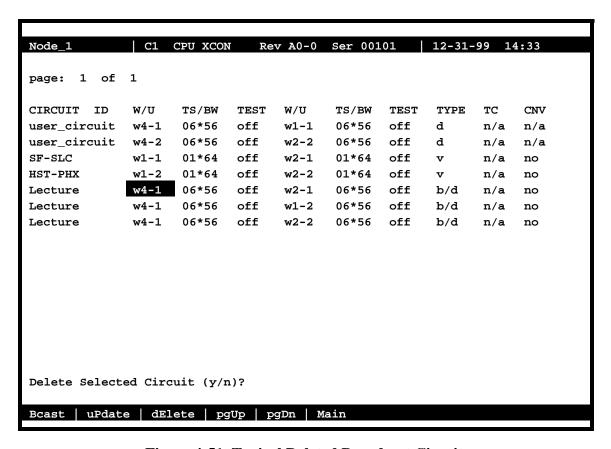
Figure 4-51. Typical Deleted Broadcast Circuit
