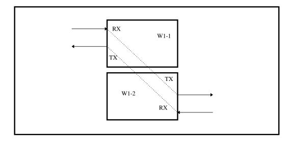
Figure 7-48. PARS Time slot Cross-connection between Primary and Secondary WANs
