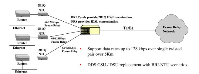
Figure 2-24. IDSL Service Provisioning
