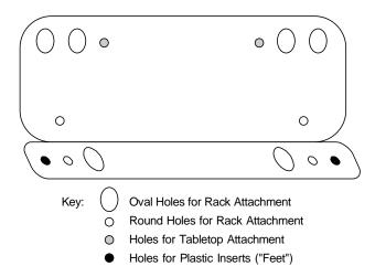
Figure 3-2. Mounting Bracket Holes
