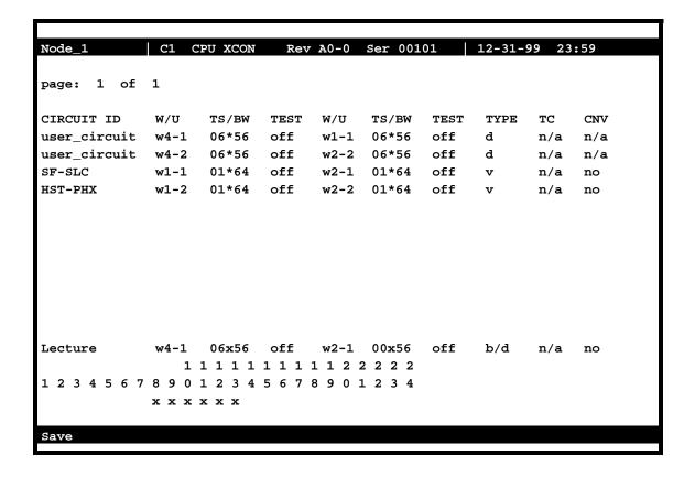
Figure 4-48. Typical Time Slot Selection
