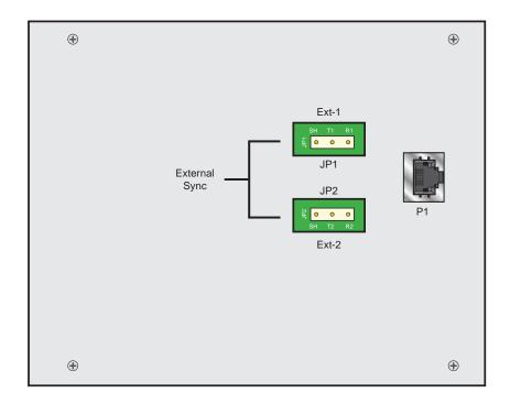
Figure 6-4. External Timing Sync Panel
