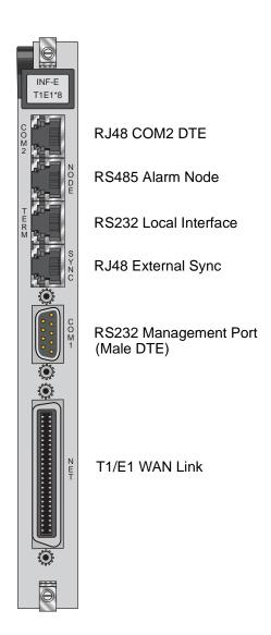
Figure C-1. INF-E Card Connectors
