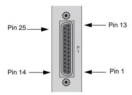
Figure C-24. HSU 35 Card Jack Pin Orientation
