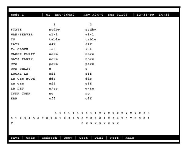
Figure 4-19. Typical HSU Card Time Slot Assignments for E1
