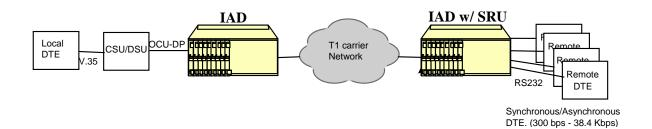
Figure 2-5. IAD with SRU Card Application
