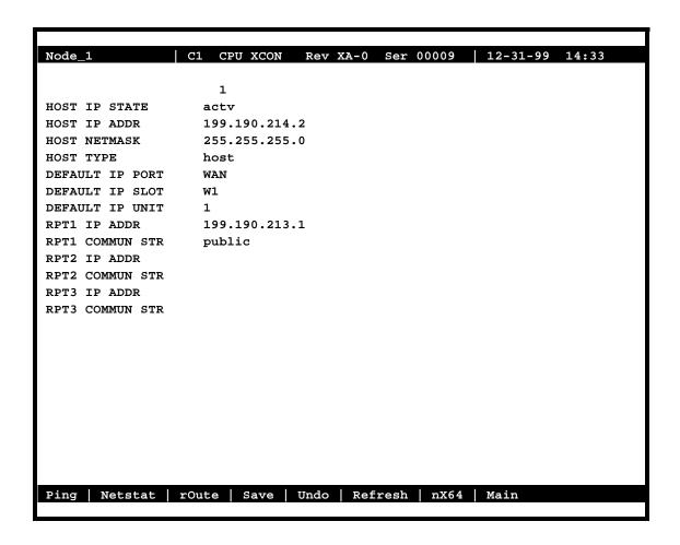
Figure 5-6. Typical TCP/IP Screen
