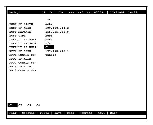
Figure 5-8. CPU Default IP Unit Selection Screen
