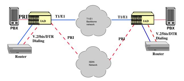
Figure 2-17. IAD using a PRI Server Card for Data Backup
