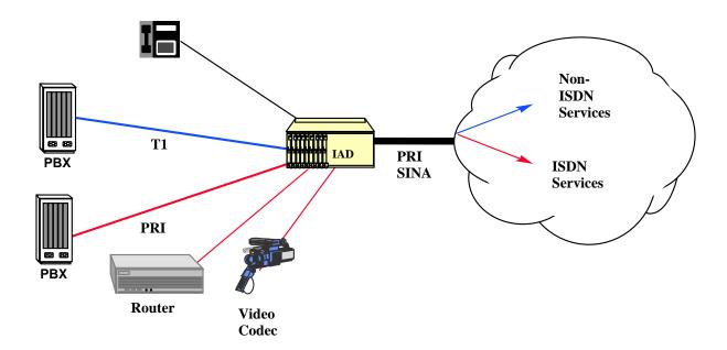
Figure 2-16. IAD using SINA for ISDN and Leased Line Traffic
