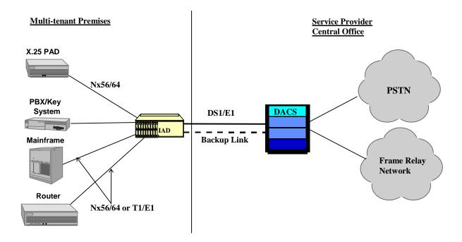
Figure 2-23. Frame Relay and Internet Services using IAD FRAD Server
