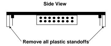
Figure 7-20. Removal of Plastic Standoffs - 811 WAN Module
