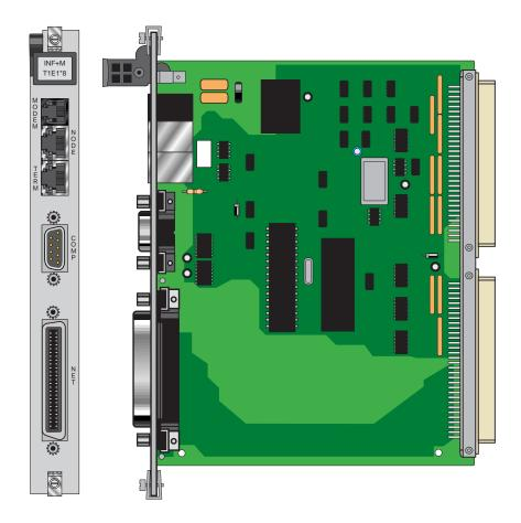
Figure 6-5. INF+M Interface Card
