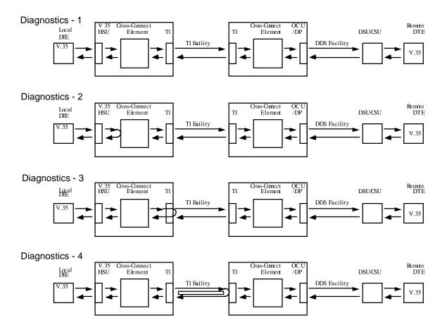
Figure 8-1. Built-In Diagnostics Example
