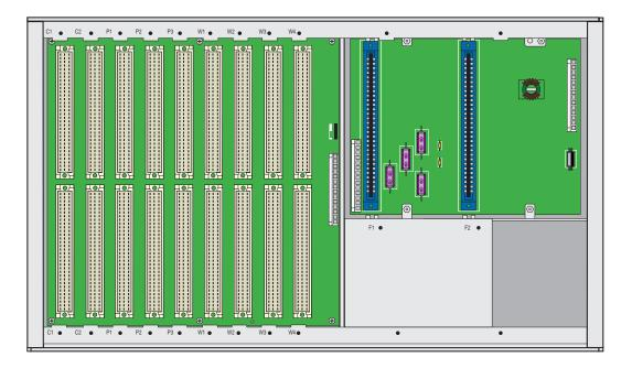
Figure 1-2. Two-Sided Chassis Front View (891830)
