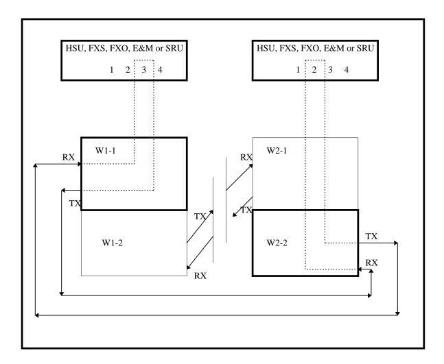
Figure 7-52. PARS Rerouting (two nodes)
