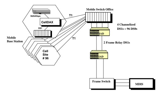
Figure 2-25. Cellular Network Frame Relay Application
