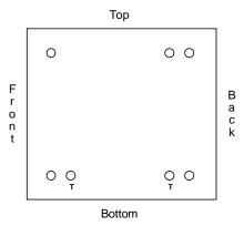
Figure 3-1. Mounting Holes for Front-Loading Chassis with Power Supplies on the Side
