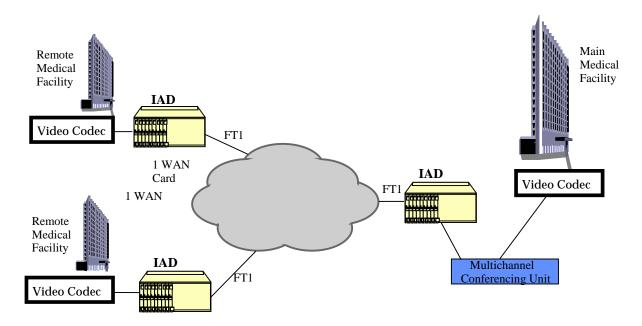
Figure 2-4. Point to MultiPoint One-Way Video and Audio using HSUs
