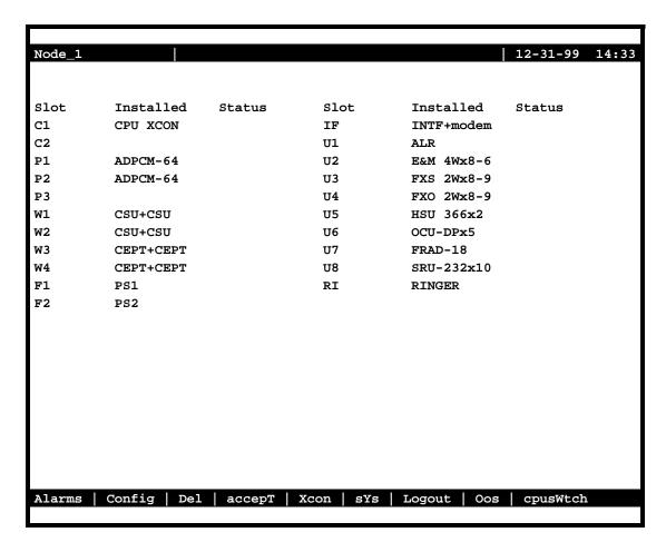
Figure 4-7. Typical System Main Screen (Two-Sided Chassis and Front-Loading Chassis with Power Supplies on Top)
