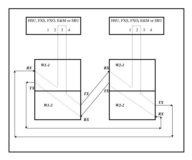
Figure 7-51. PARS Normal Operation Mode (two nodes)
