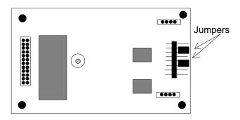
Figure 7-10. DSX/CEPT Revision E+ Module Jumpers
