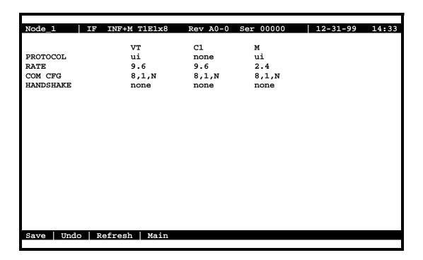
Figure 6-11. Typical Ports Screen (INTF+M)
