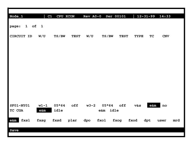
Figure 4-32. Trunk Conditioning Option Selection
