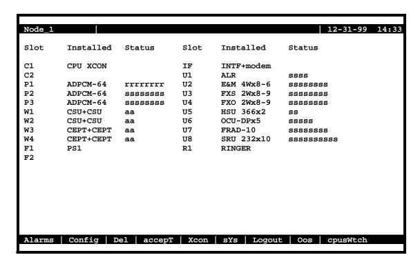
Figure 4-70. Typical ADPCM Card Redundancy Switch in Progress
