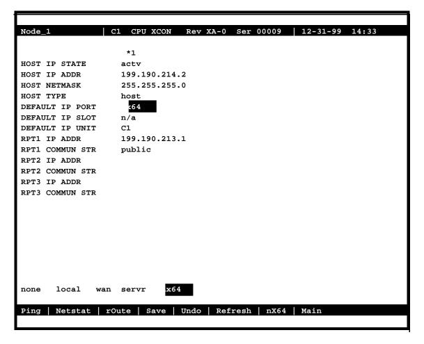
Figure 5-7. CPU Default IP Port Selection Screen
