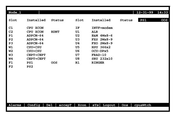
Figure 4-62. Typical Redundant-Power Supply System Main Screen
