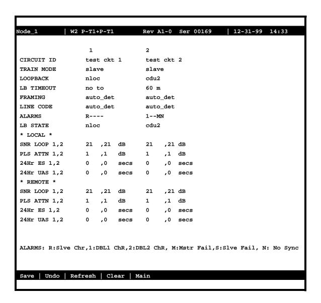
Figure 7-37. PairGain T1/HDSL Module Screen
