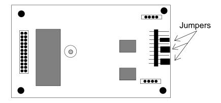
Figure 7-15. DSX/CEPT Revision A1 to D1 Module Jumpers
