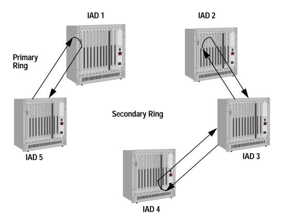
Figure 7-47. Traffic Flow when two connected IADs are separated from the Ring
