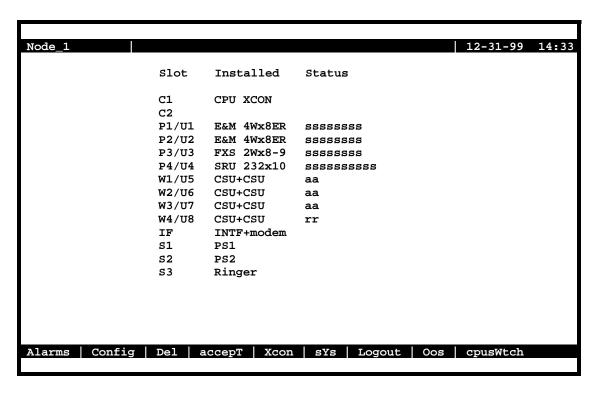
Figure 4-65. Typical Cross-Connect System with WAN Card Redundancy
