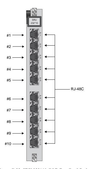
Figure C-33. SRU 232\*10 C&D Bus Card Jacks
