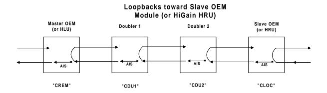
Figure 7-39. PairGain T1/HDSL System Loopbacks towards Slave Module
