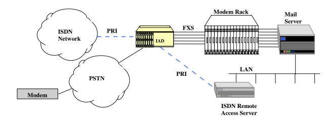
Figure 2-18. PRI to FXS Termination
