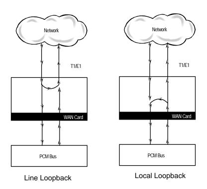
Figure 7-24. Line and Local Loopbacks
