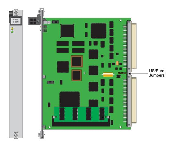
Figure 5-1. CPU XCON US/EURO Jumper Settings
