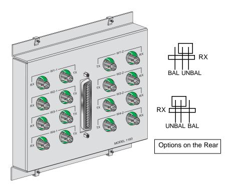
Figure 7-21. E1 Interface Adapter Panel
