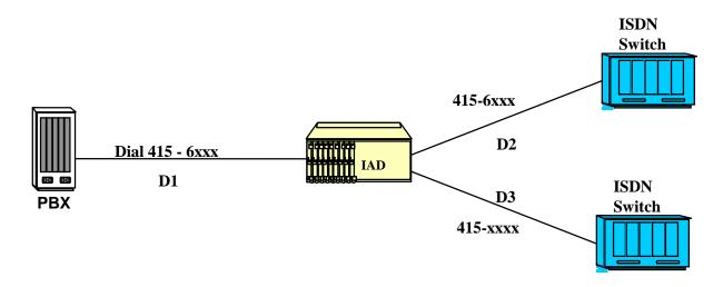
Figure 2-20. Alternate Routing
