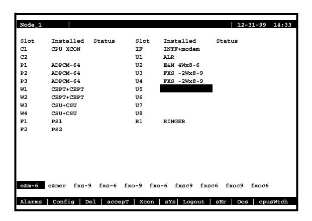
Figure 4-21. Typical Card Slot and Type Selection
