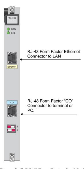
Figure C-45. RJ-48 Form Factor Card Jacks
