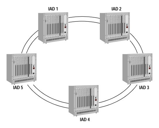
Figure 7-44. Ring Network Traffic Flow
