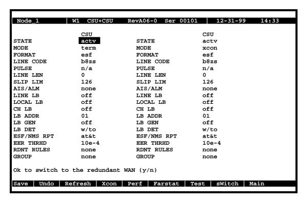
Figure 4-66. Switching to a Redundant Cross-Connect WAN Card
