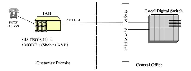
Figure 2-2. IAD using TR008
