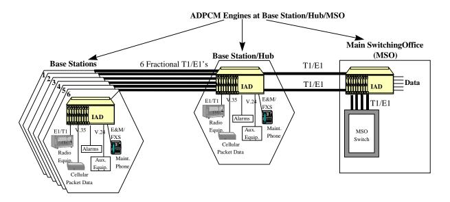
Figure 2-12. IAD in a Wireless Base Station Application
