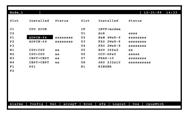
Figure 4-68. Typical System with Redundant ADPCM Cards
