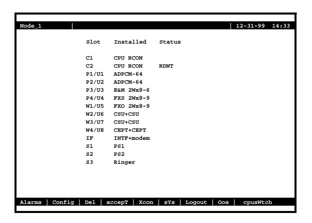
Figure 4-8. Typical System Main Screen (Front-Loading Chassis with Power Supplies on the Side)
