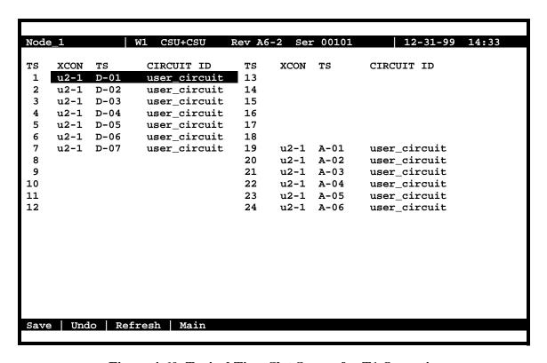
Figure 4-60. Typical Time Slot Screen for T1 Operation
