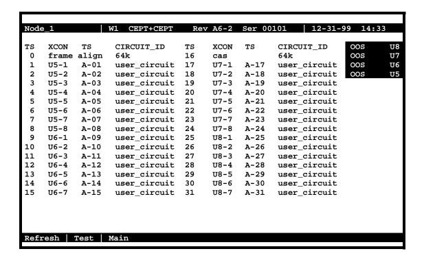
Figure 4-24. Typical WAN Time Slot Assignment Screen
