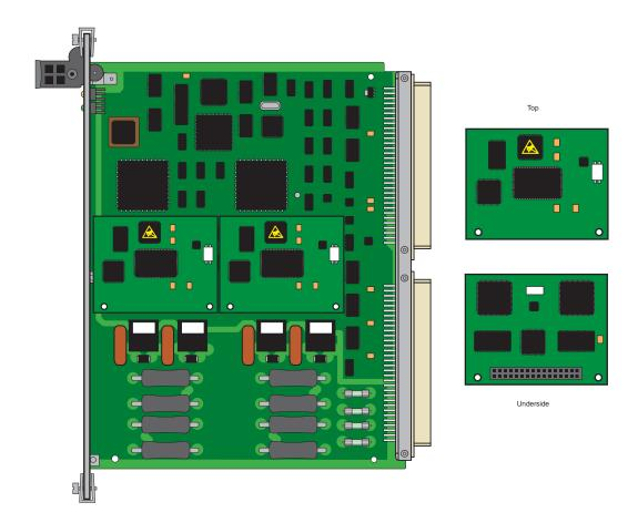
Figure 7-22. WAN HDSL Card with PairGain T1/HDSL Modules
