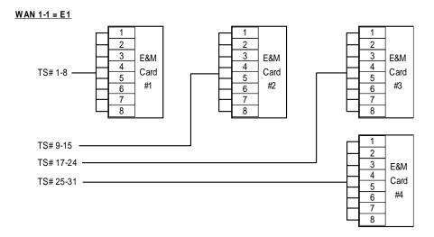
Figure 4-20. Automatic Time Slot Assignment Example
