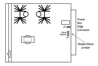
Figure 3-7. 105V Ringing Generator Jumper Setting
