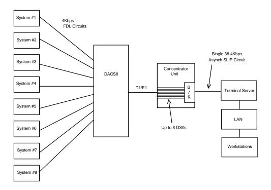
Figure 5-5. Typical TCP/IP Network Management System
