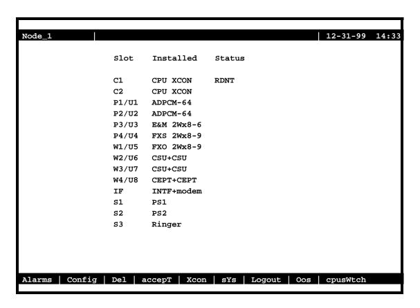
Figure 4-64. Typical System with CPU Switchover Completed
