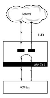
Figure 7-25. DS0 Time Slot Loopback
