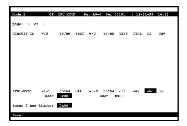
Figure 4-33. Signaling Bit Pattern Selection
