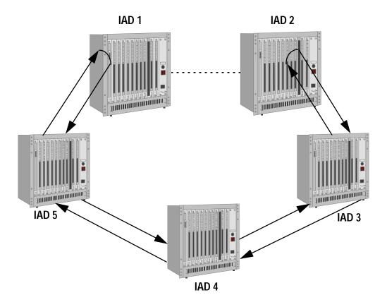
Figure 7-45. Traffic Flow when One Link is Lost
