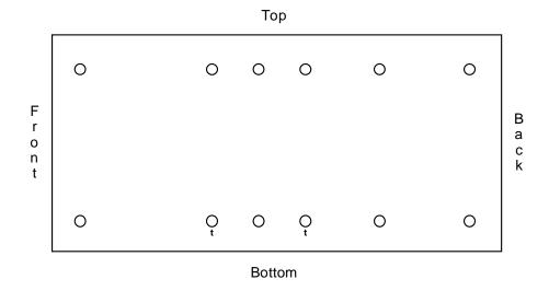
Figure 3-4. Two-Sided Chassis Mounting Holes
