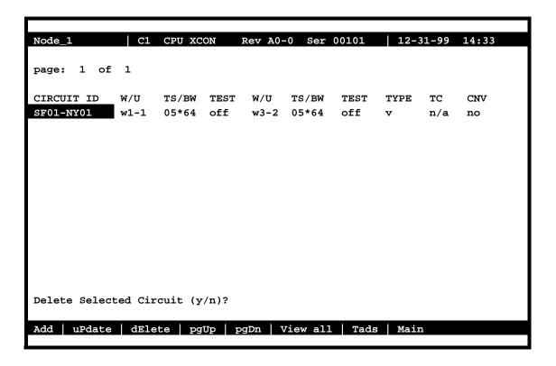
Figure 4-39. Delete Cross-Connection Screen
