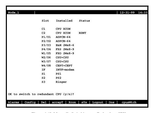
Figure 4-63. Manually Switching to a Redundant CPU
