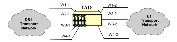
Figure 2-3. IAD using T1/E1 Conversion
