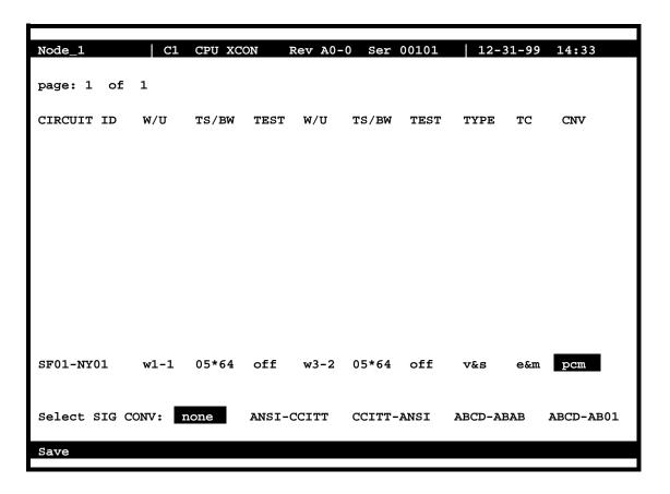
Figure 4-36. Selecting Signaling Conversion
