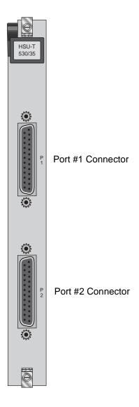
Figure C-28. HSU-T V35 Card Front Panel Connectors
