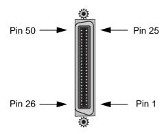
Figure C-31. Four-Port HSU\*4E 530/35 Card Jacks
