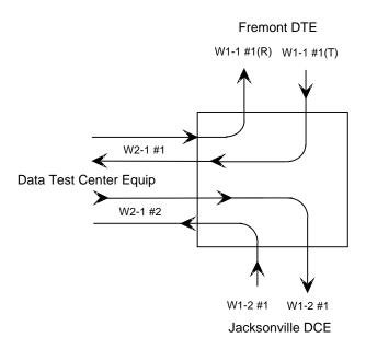
Figure 4-57. Split Circuit Diagram
