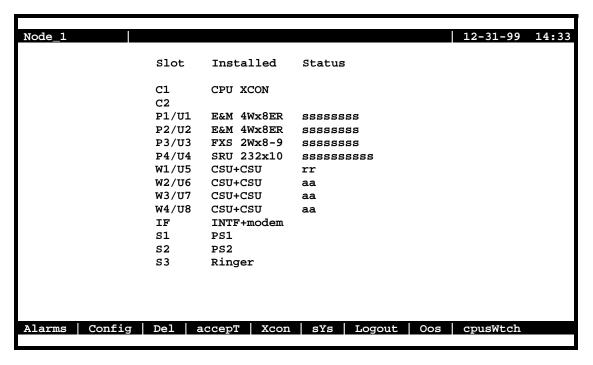
Figure 4-67. Typical Cross-Connect WAN Card Redundancy Switch in Progress
