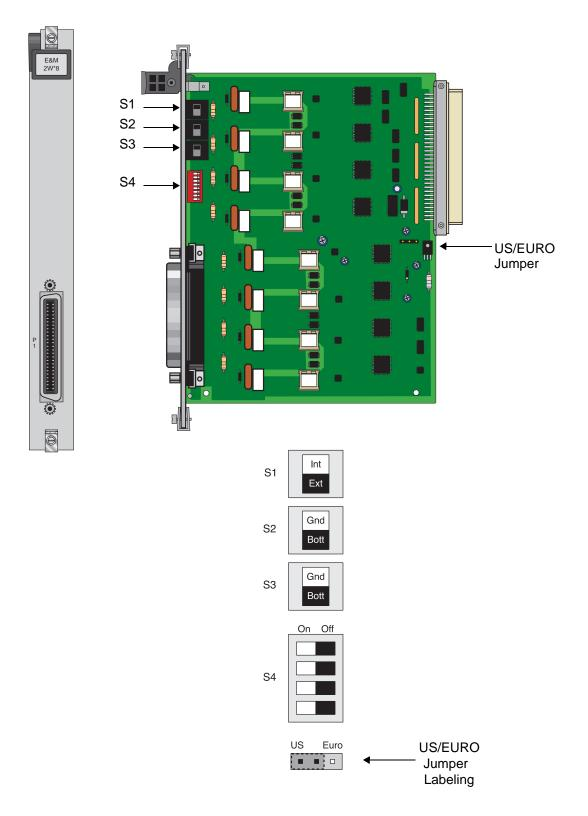
Figure 1-1. Typical E&M Card Switches
