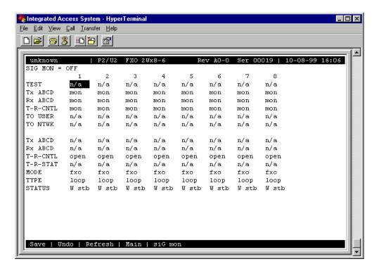
Figure 3-4. Typical FXO Card Test Screen
