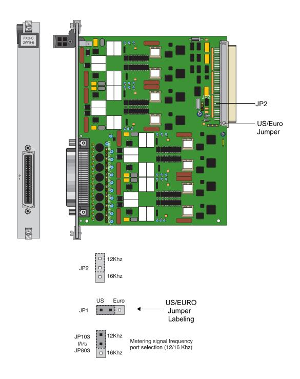
Figure 5-1. Jumpers for MRD Mode
