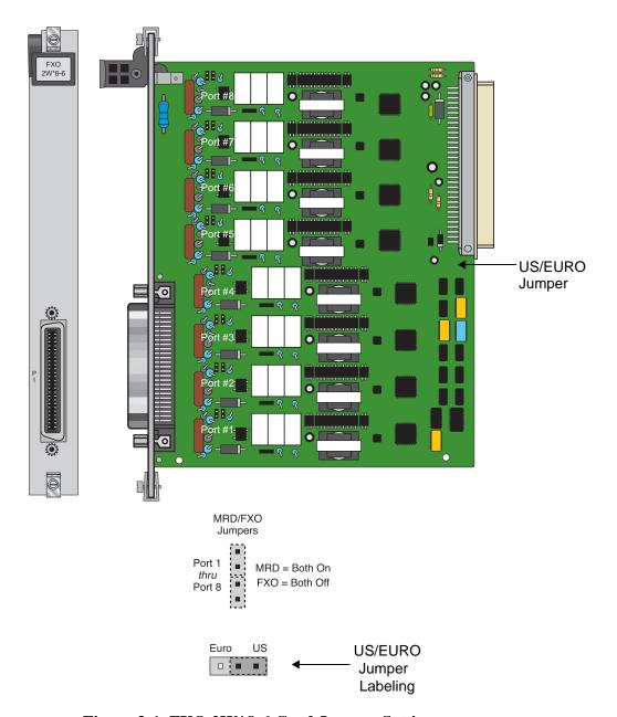
Figure 3-1. FXO 2W\*8-6 Card Jumper Settings
