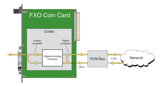
Figure 5-3. FXO Coin Card Loopbacks
