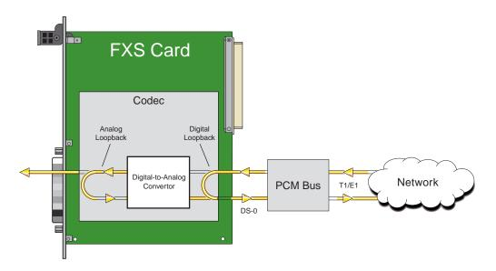
Figure 2-3. FXS Card Loopbacks
