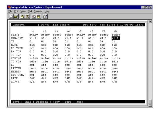
Figure 1-2. Typical E&M Card Main Screen
