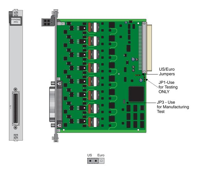
Figure 7-1. P-Phone PPO and PPS Cards Jumper Settings
