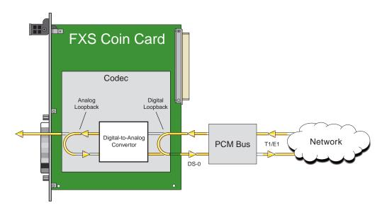
Figure 4-3. FXS Coin Card Loopbacks
