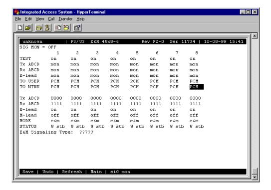
Figure 1-4. Typical E&M Card Test Screen
