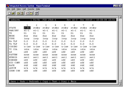
Figure 2-2. Typical FXS Card Main Screen
