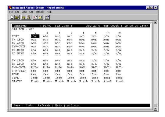
Figure 2-4. Typical FXS Card Test Screen
