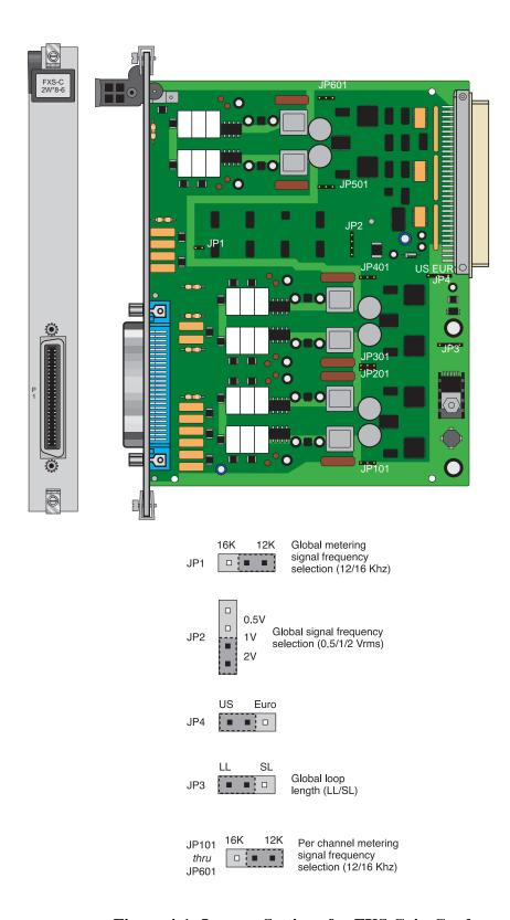
Figure 4-1. Jumper Settings for FXS Coin Card
