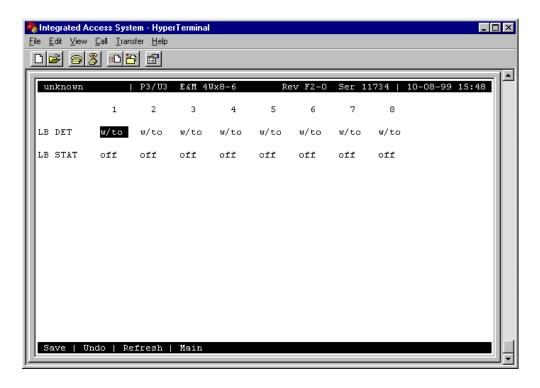
Figure 1-5. Typical E&M Loopback Screen
