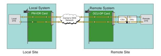
Figure 8-7. Remote CSU Loopback
