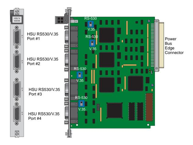
Figure 1-4. Four-Port HSU 530/35 Card Switches
