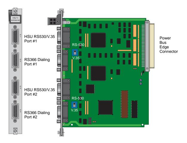
Figure 1-2. HSU-AD 530/35 Card Switches
