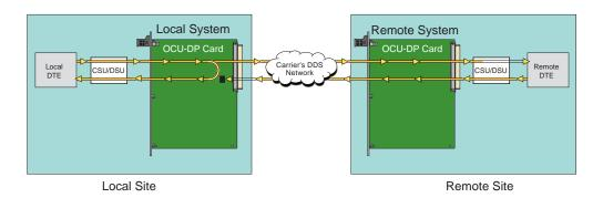
Figure 3-3. OCU Local Loopback (dte option)
