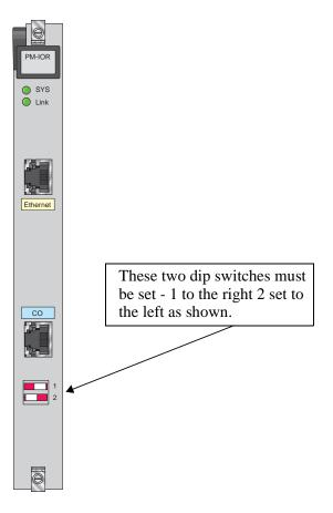
Figure 8-1. PM-IOR Card Dip-switch settings (828060)
