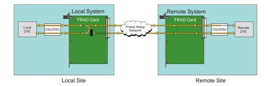
Figure 4-3. DTE Loopback
