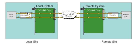
Figure 3-8. OCU Remote Loopback (csu-u option)
