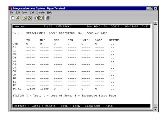
Figure 1-22. Typical HSU Performance Data Screen
