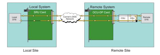
Figure 2-8. Inband Remote DSU Loopback
