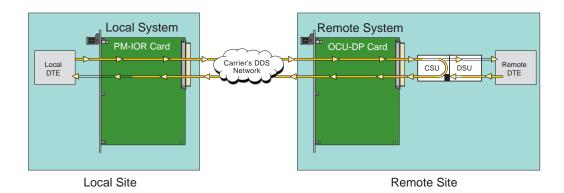
Figure 8-8. Remote DSU Loopback
