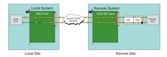
Figure 1-14. Remote DSU Loopback
