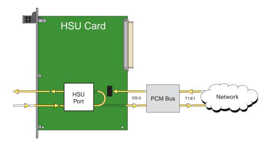
Figure 1-10. Local DTE Loopback
