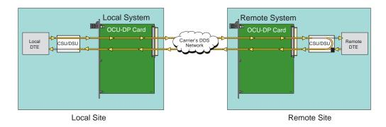
Figure 3-7. OCU Remote Loopback (csu-n option)
