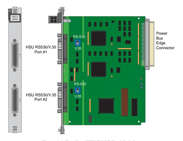
Figure 1-1. Two-Port HSU 530/35 Card Switches
