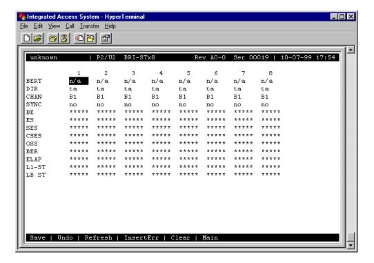
Figure 7-18. Typical BRI-ST\*8 Card Test Screen
