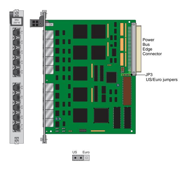
Figure 2-1. SRU 232\*10 Jumper Settings
