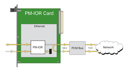
Figure 8-4. Local DTE Loopback
