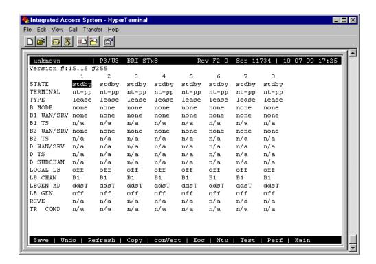
Figure 7-7. Typical BRI-ST\*8 Card Main Screen
