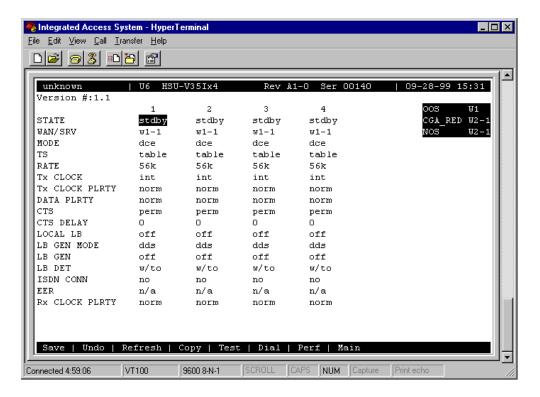
Figure 1-8. Typical HSU Card Main Screen
