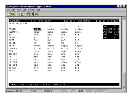
Figure 2-3. Typical SRU Card Main Screen
