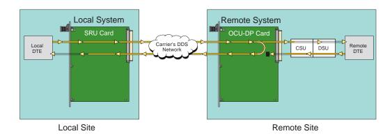
Figure 2-6. Inband Remote SRU Loopback
