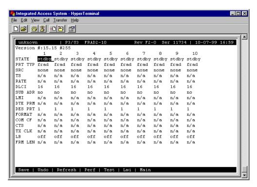
Figure 4-2. Typical FRAD Card Main Screen
