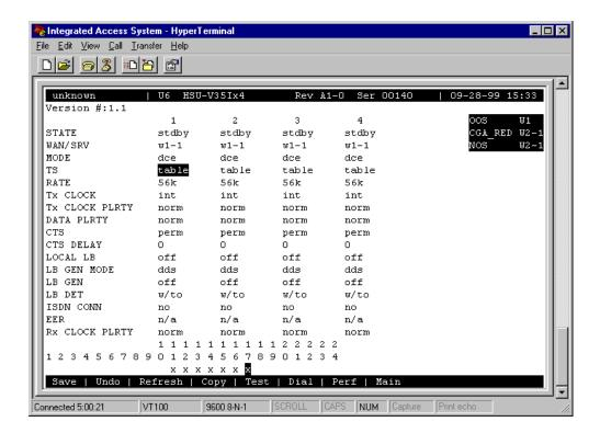
Figure 1-9. Typical HSU Port Time Slot Assignment Screen
