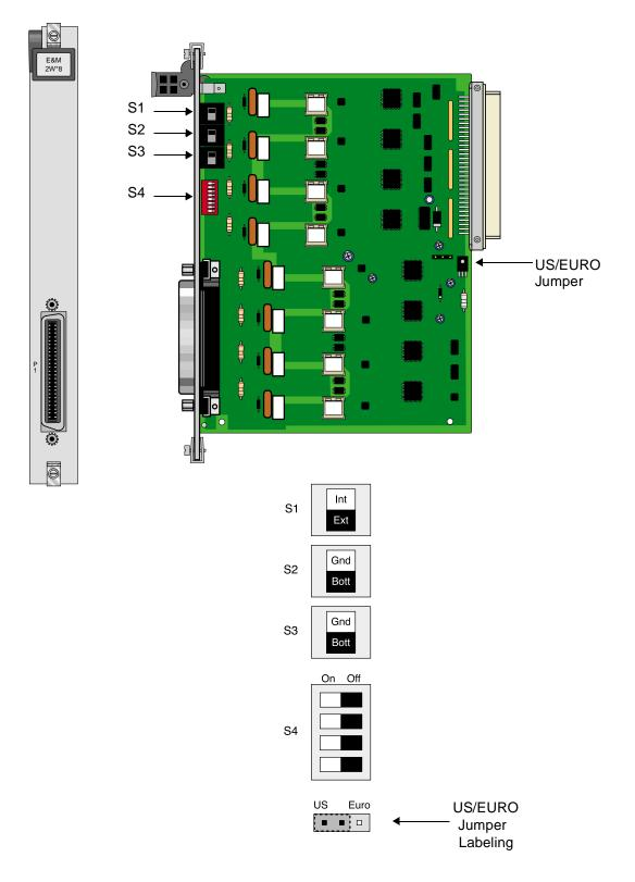
Figure 1-1. Typical E&M Card Switches
