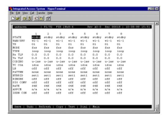
Figure 2-2. Typical FXS Card Main Screen
