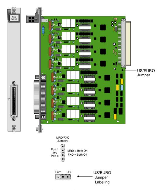
Figure 3-1. FXO 2W\*8-6 Card Jumper Settings
