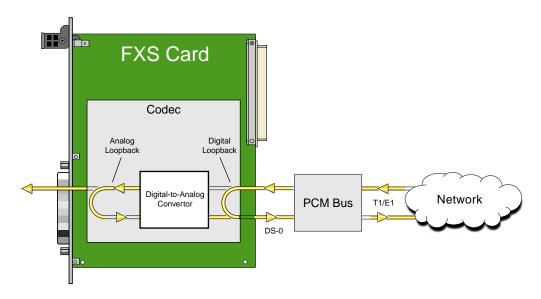
Figure 2-3. FXS Card Loopbacks
