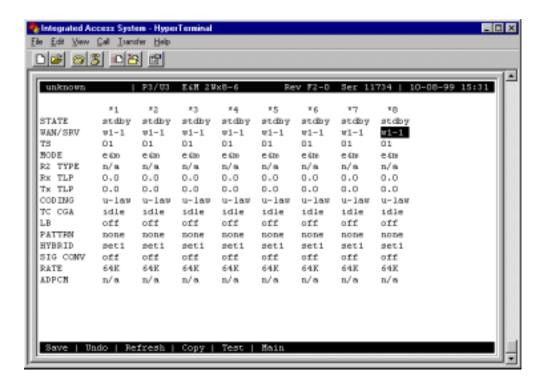
Figure 1-2. Typical E&M Card Main Screen
