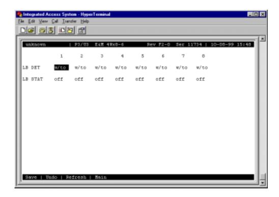
Figure 1-5. Typical E&M Loopback Screen
