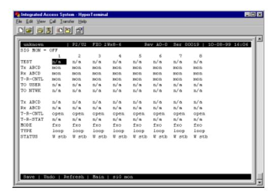
Figure 3-4. Typical FXO Card Test Screen
