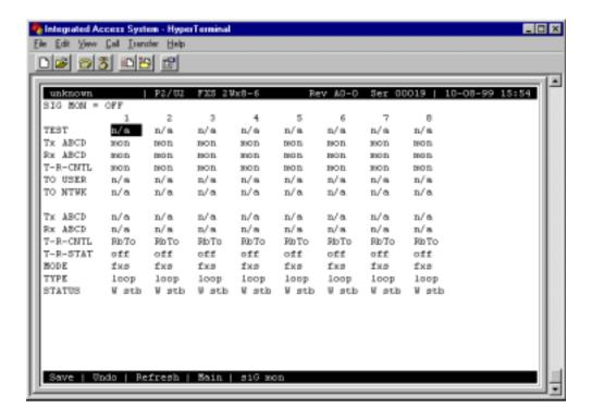
Figure 2-4. Typical FXS Card Test Screen
