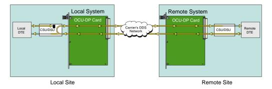
Figure 3-8. OCU Remote Loopback (csu-u option)
