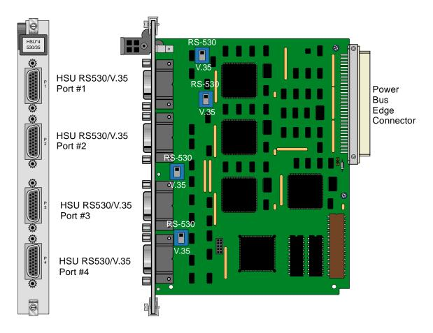
Figure 1-4. Four-Port HSU 530/35 Card Switches
