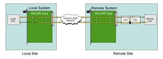
Figure 6-7. Remote CSU Loopback
