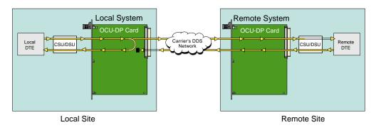
Figure 3-3. OCU Local Loopback (dte option)
