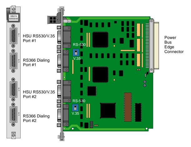
Figure 1-2. HSU-AD 530/35 Card Switches
