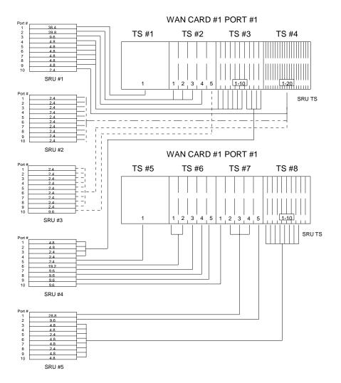
Figure 2-9. Typical WAN Time Slot Assignments to an SRU Card
