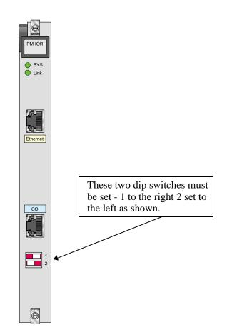
Figure 6-1. PM-IOR Card Dip-switch settings (828060)
