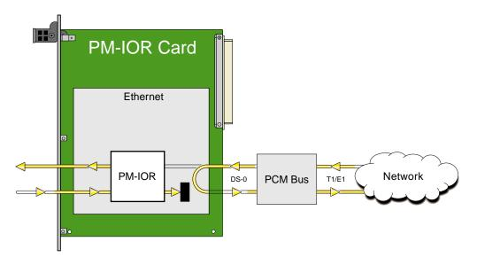
**Figure 6-4. Local DTE Loopback**
