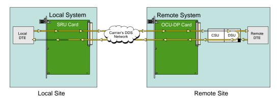
Figure 2-8. Inband Remote DSU Loopback
