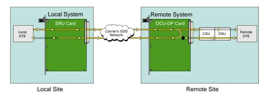
Figure 2-6. Inband Remote SRU Loopback
