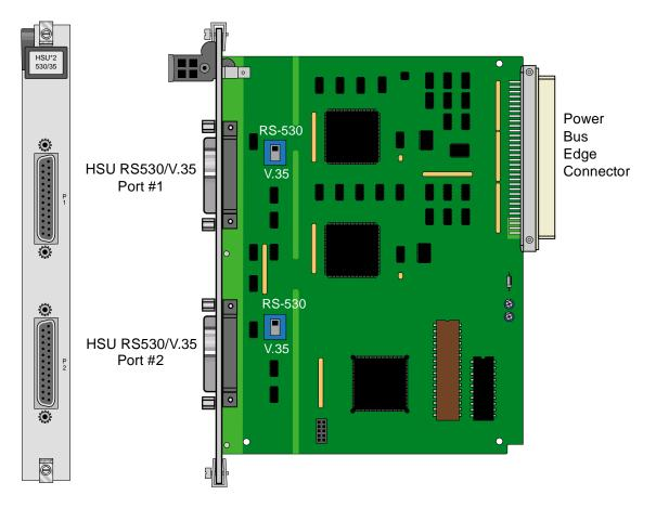
Figure 1-1. Two-Port HSU 530/35 Card Switches
