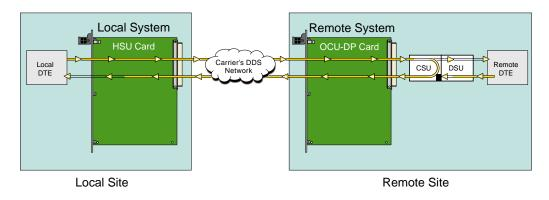
Figure 1-13. Remote CSU Loopback
