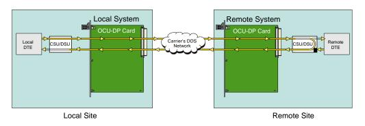
Figure 3-7. OCU Remote Loopback (csu-n option)
