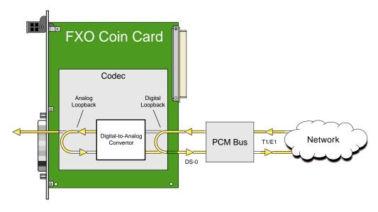
Figure 5-3. FXO Coin Card Loopbacks
