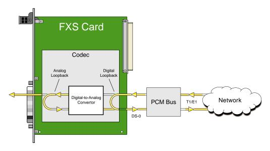
Figure 2-3. FXS Card Loopbacks
