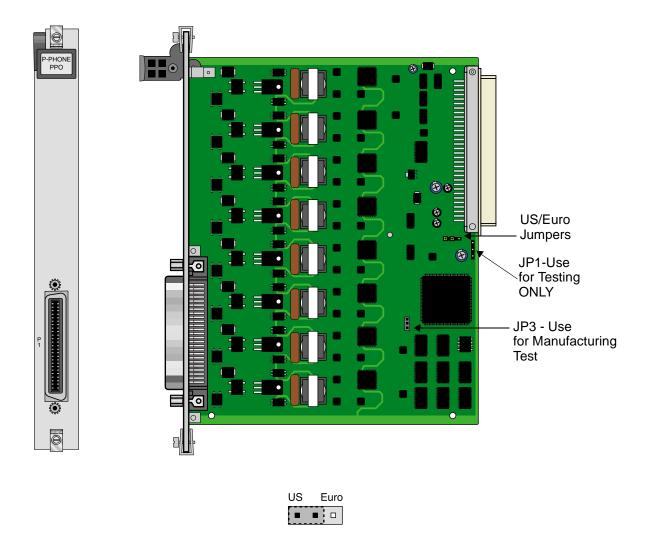
Figure 7-1. P-Phone PPO and PPS Cards Jumper Settings
