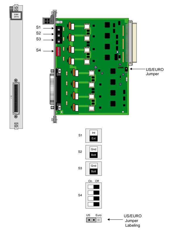
Figure 1-1. Typical E&M Card Switches
