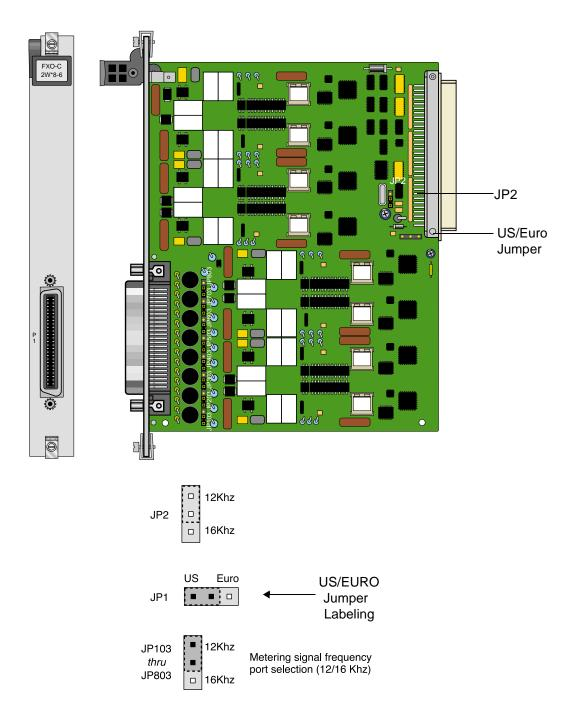
Figure 5-1. Jumpers for MRD Mode
