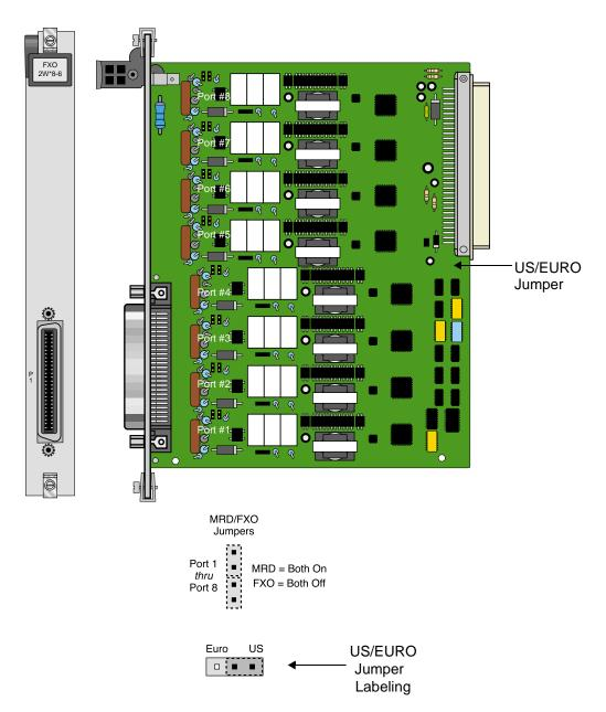
Figure 3-1. FXO 2W\*8-6 Card Jumper Settings
