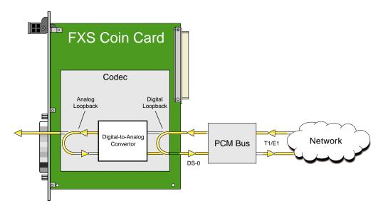
Figure 4-3. FXS Coin Card Loopbacks
