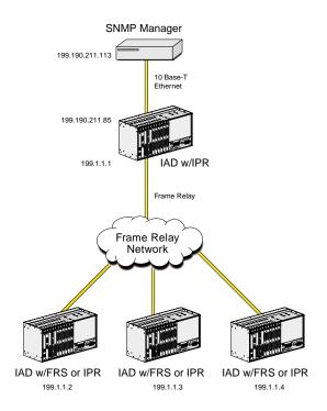
Figure 8-3. IPR Card Connected to IP Nodes on Ethernet to Frame Relay Network
