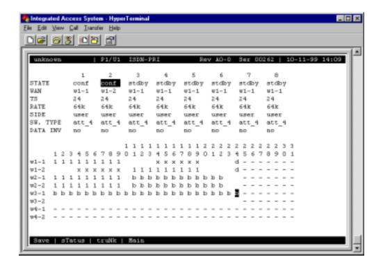
Figure 6-13. Assigning B Channels
