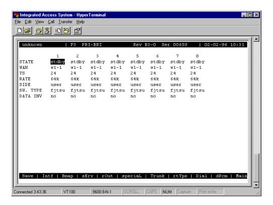
Figure 6-8. D Channel Configuration Screen
