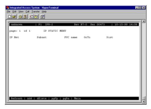
Figure 8-19. IPR 10B2 and 10BT IP Static Routes Configuration Menu Screen
