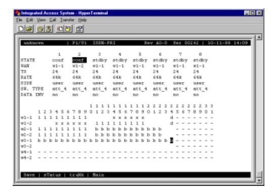
Figure 5-13. Assigning B Channels
