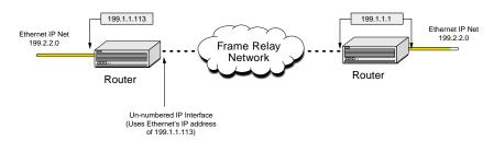
Figure 8-8. Unnumbered Frame Relay IP Interface
