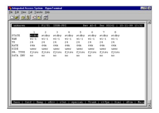
Figure 5-8. D Channel Configuration Screen
