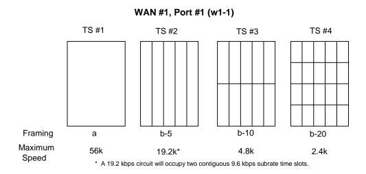
Figure 3-2. Data Frames, Rates, and Time Slot Assignments
