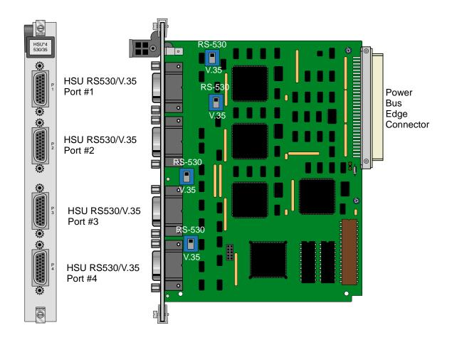
Figure 1-4. Four-Port HSU 530/35 Card Switches
