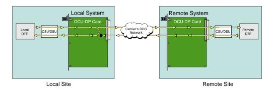
Figure 3-3. OCU Local Loopback (dte option)
