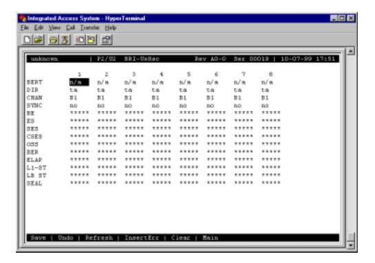
Figure 7-17. Typical BRI-U\*8 and BRI-SC U\*8 Card Test Screen
