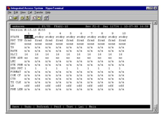
Figure 4-2. Typical FRAD Card Main Screen
