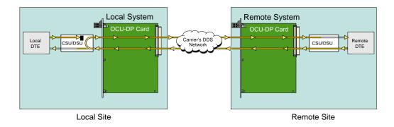
Figure 3-8. OCU Remote Loopback (csu-u option)
