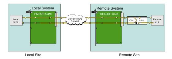
Figure 8-7. Remote CSU Loopback
