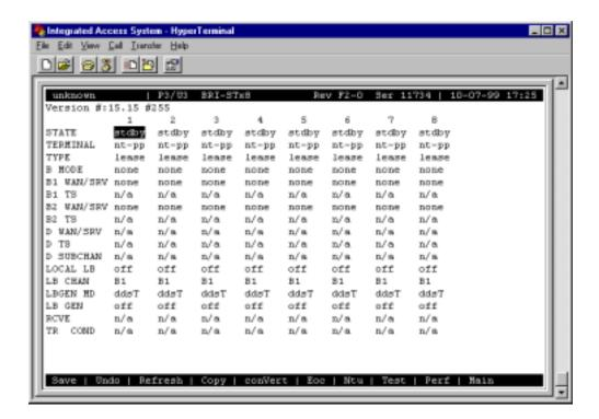
Figure 7-7. Typical BRI-ST\*8 Card Main Screen
