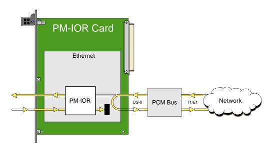
Figure 8-4. Local DTE Loopback
