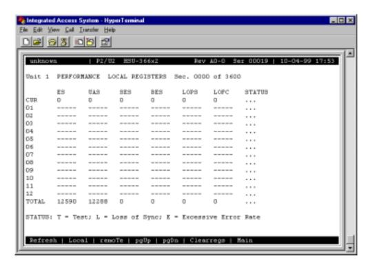
Figure 1-22. Typical HSU Performance Data Screen
