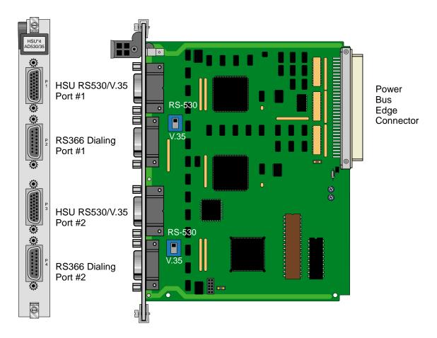
Figure 1-2. HSU-AD 530/35 Card Switches
