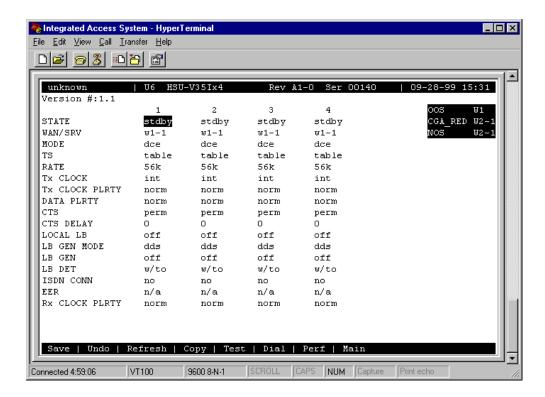
Figure 1-8. Typical HSU Card Main Screen
