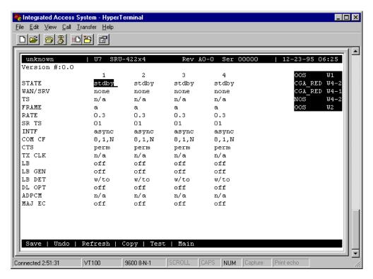
Figure 2-3. Typical SRU Card Main Screen
