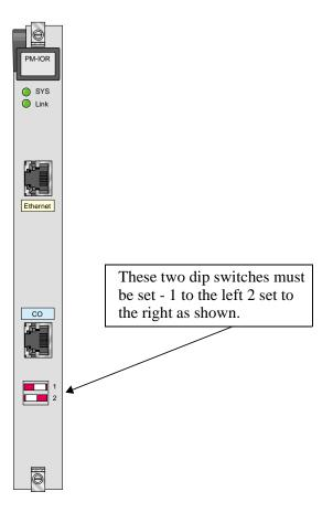
Figure 8-1. PM-IOR Card Dip-switch settings (828060)
