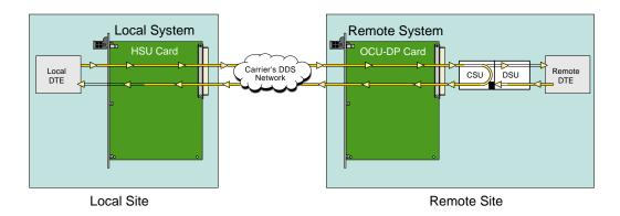
Figure 1-13. Remote CSU Loopback
