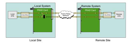
Figure 4-3. DTE Loopback
