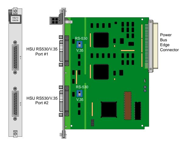
Figure 1-1. Two-Port HSU 530/35 Card Switches
