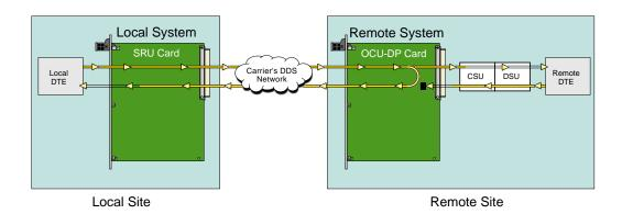
Figure 2-6. Inband Remote SRU Loopback
