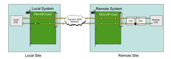
Figure 8-8. Remote DSU Loopback
