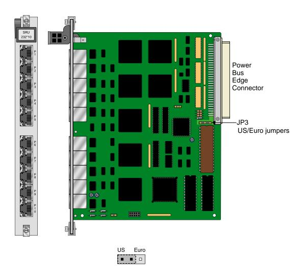
Figure 2-1. SRU 232\*10 Jumper Settings
