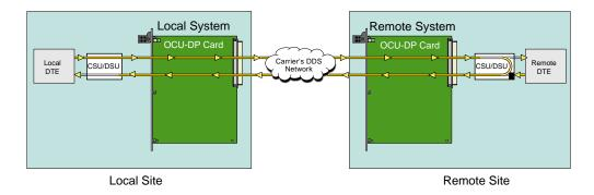
Figure 3-7. OCU Remote Loopback (csu-n option)
