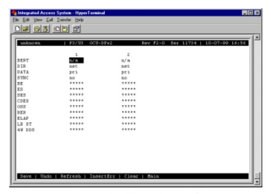
Figure 3-10. Typical OCU-DP Card Test Screen
