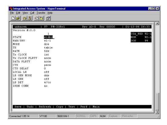
Figure 8-2. Typical PM-IOR Card Main Screen
