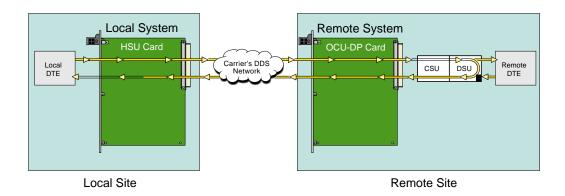
Figure 1-14. Remote DSU Loopback
