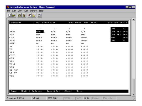
Figure 2-10. Typical SRU Card Test Screen
