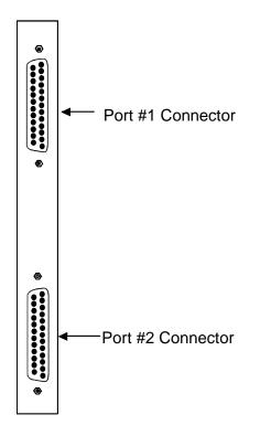
Figure C-28. HSU-T V35 Card Front Panel Connectors
