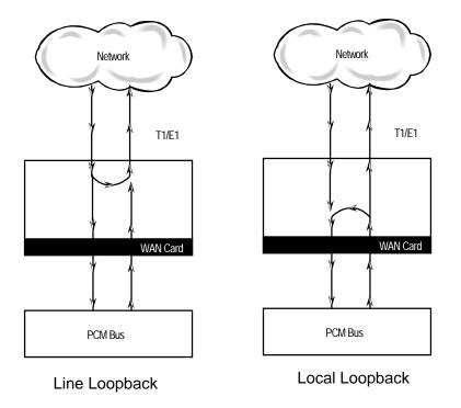
Figure 6-21. Line and Local Loopbacks
