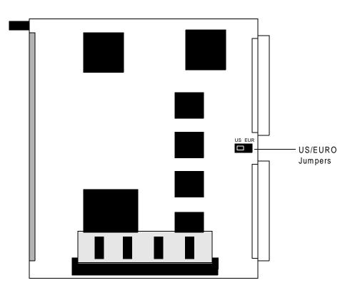
Figure 4-1. CPU XCON US/EURO Jumper Settings
