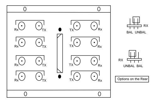
Figure 6-19. E1 Interface Adapter Panel
