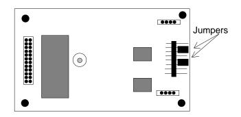
Figure 6-8. DSX/CEPT Revision E+ Module Jumpers
