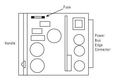
Figure 2-6. -48V Converter Fuse
