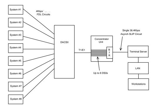
Figure 4-5. Typical TCP/IP Network Management System
