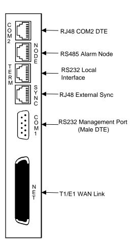
**Figure C-1. INF-E Card Connectors**
