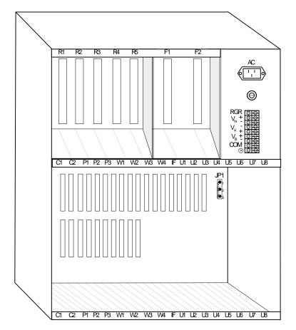
Figure 1-5. Front-Loading Chassis with Power Supplies on Top
