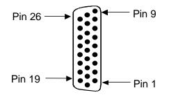
Figure C-26. HSU-AD 530/35 Card Jack Pin Orientation
