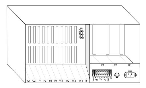
Figure 1-2. Front-Loading Chassis (six-digit) with Power Supplies on Side
