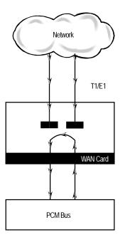
Figure 6-22. DS0 Time Slot Loopback
