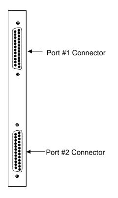
Figure C-21. Two-Port HSU 530/35 Front Panel Connectors
