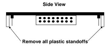
Figure 6-18. Removal of Plastic Standoffs - 811 WAN Module
