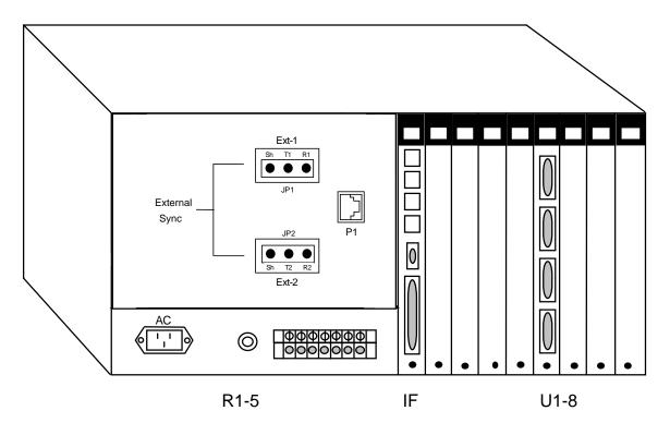
Figure 5-2. Two-Sided Chassis, Back View with External Sync Panel Installed
