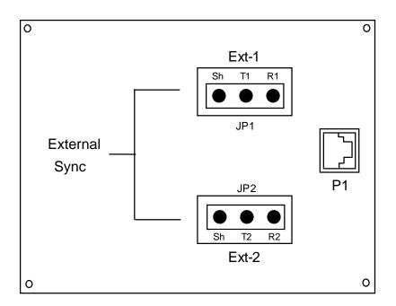
**Figure 5-3. External Timing Sync Connection**
