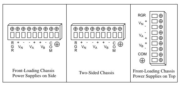
Key: 🔁 = Chassis Ground COM = Common System Ground
