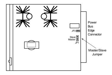
Figure 2-7. 105V Ringing Generator Jumper Setting
