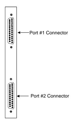
Figure C-23. HSU-T V11 Card Front Panel Connectors
