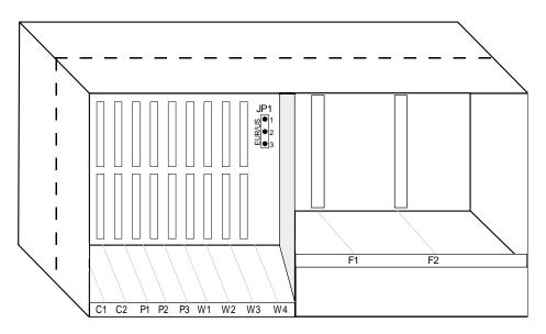
Figure 1-3. Two-Sided Chassis Front View
