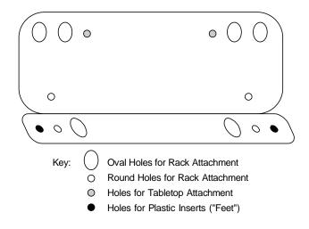
**Figure 2-2. Mounting Bracket Holes**
