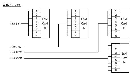
Figure 3-22. Automatic Time Slot Assignment Example
