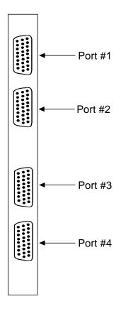
Figure C-30. Four-Port HSU 530/35 Card Jacks
