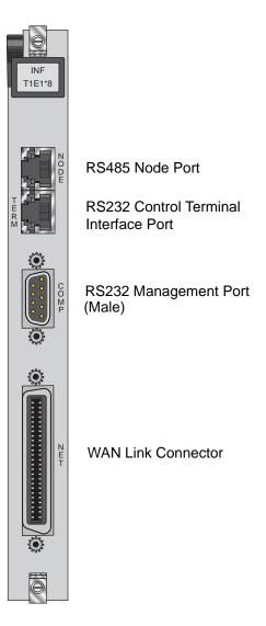
Figure C-7. INF T1E1\*8 Interface Card Jacks
