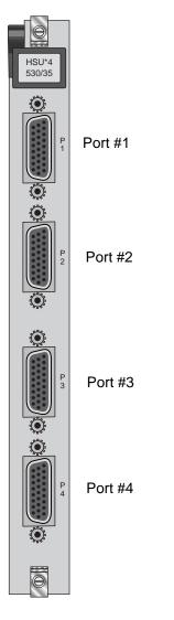
Figure C-26. Four-Port HSU 530/35 Card Jacks
