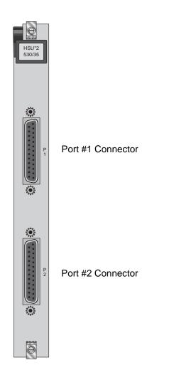
Figure C-17. Two-Port HSU 530/35 Front Panel Connectors
