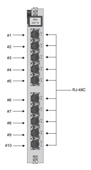
Figure C-29. SRU 232\*10 C&D Bus Card Jacks
