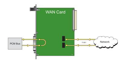
Figure 7-24. DS0 Time Slot Loopback
