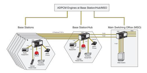
Figure 2-12. IAD in a Wireless Base Station Application
