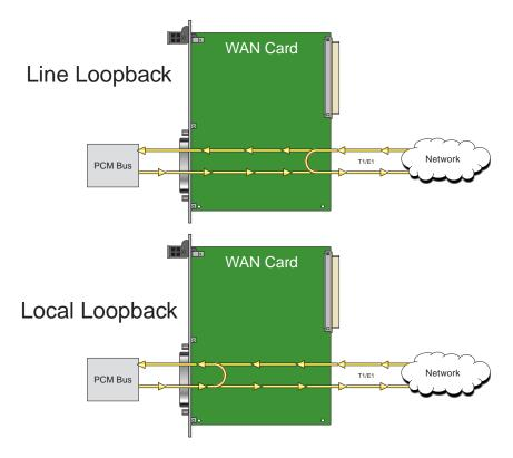
Figure 7-23. Line and Local Loopbacks
