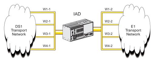
Figure 2-3. IAD using T1/E1 Conversion
