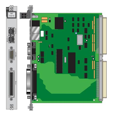
Figure 6-2. INF T1E1\*8 Interface Card
