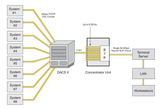
Figure 5-7. Typical TCP/IP Network Management System
