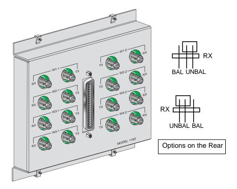
Figure 7-21. E1 Interface Adapter Panel
