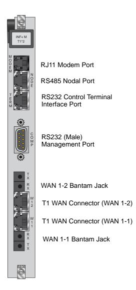
Figure C-11. INF+M T1\*2 Interface Card Jacks
