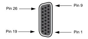
Figure C-22. HSU-AD 530/35 Card Jack Pin Orientation
