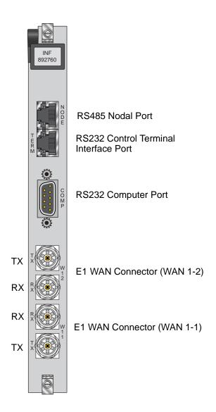
Figure C-12. INF E1\*2 Interface Card Jacks
