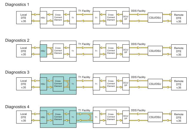
Figure 8-1. Built-In Diagnostics Example
