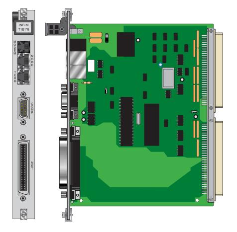
Figure 6-1. INF+M T1E1\*8 Interface Card
