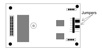
Figure 7-10. DSX/CEPT Revision E+ Module Jumpers
