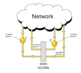
Figure 4-45. Voice Test Diagram
