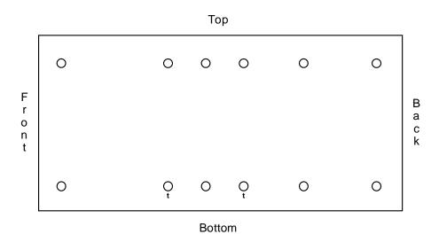
Figure 3-4. Two-Sided Chassis Mounting Holes
