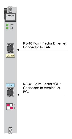
Figure C-41. RJ-48 Form Factor Card Jacks
