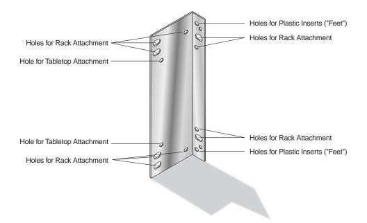
**Figure 3-2. Mounting Bracket Holes**
