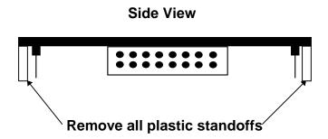
Figure 7-20. Removal of Plastic Standoffs - 811 WAN Module
