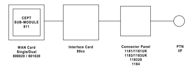
The Interface Card is also listed in the approval documentation and provides a direct metallic path between the CEPT module and appropriate Connector Panel.
