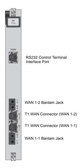
Figure C-10. INF T1\*2 Interface Card Jacks
