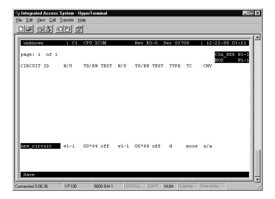
Figure 4-28. Add a Cross-Connect Circuit Screen
