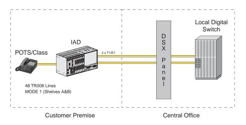
Figure 2-2. IAD using TR008
