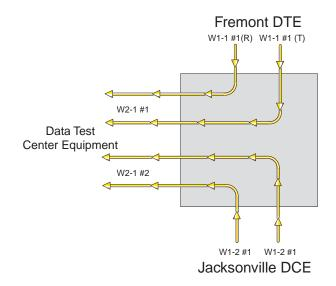
Figure 4-59. Split Circuit Diagram
