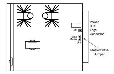
Figure 3-7. 105V Ringing Generator Jumper Setting
