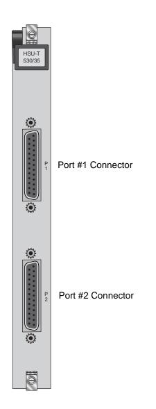
Figure C-24. HSU-T V35 Card Front Panel Connectors
