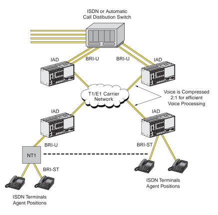
Figure 2-11. IAD in an ISDN-based ACD System
