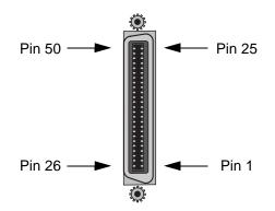
Figure C-27. Four-Port HSU\*4E 530/35 Card Jacks
