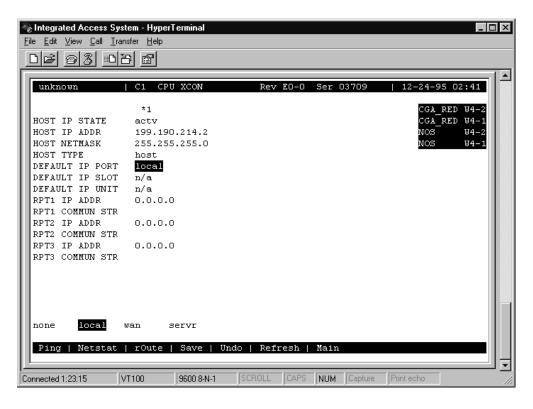
Figure 5-9. CPU Default IP Port Selection Screen
