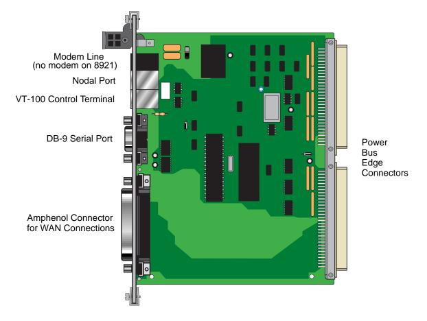
Figure 6-10. Component Layout for the INF+M T1E1\*8 and INF T1E1\*8 Interface Card
