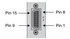
Figure C-23. HSU-AD 530/35 Card RS-366 Jack Pin Orientation
