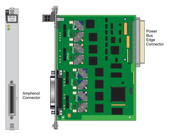
Figure 7-3. BRI-SC U\*8 Card Sealing Current Jumpers
