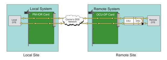
Figure 8-8. Remote DSU Loopback
