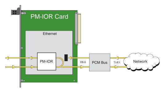
Figure 8-4. Local DTE Loopback
