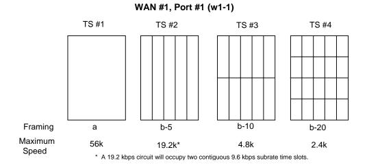
Figure 3-2. Data Frames, Rates, and Time Slot Assignments
