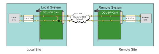
Figure 3-3. OCU Local Loopback (dte option)
