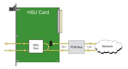
**Figure 1-10. Local DTE Loopback**
