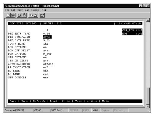
Figure 7-10. Typical Remote NTU Configuration Screen
