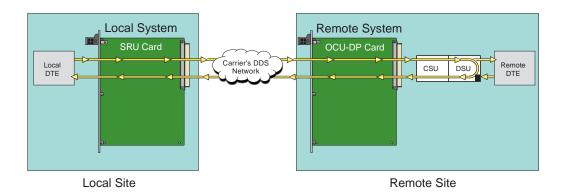
Figure 2-10. Inband Remote DSU Loopback
