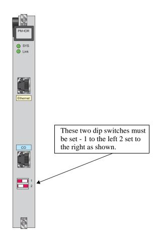
Figure 8-1. PM-IOR Card Dip-switch settings
