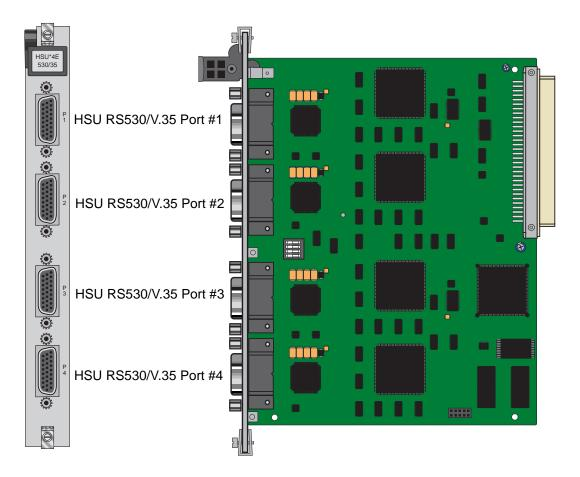
Figure 1-5. Four-Port HSU\*4E 530/35 Card Switches
