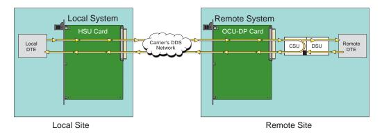
Figure 1-13. Remote CSU Loopback
