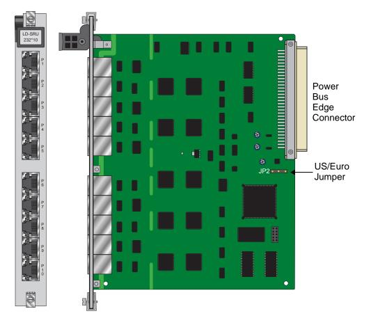
Figure 2-4. SRU-LD\*10 Card Jumper Settings
