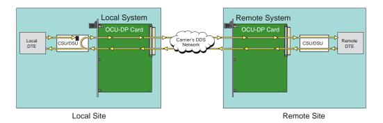
Figure 3-8. OCU Remote Loopback (csu-u option)
