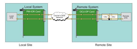
Figure 8-7. Remote CSU Loopback
