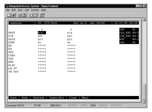
Figure 3-10. Typical OCU-DP Card Test Screen
