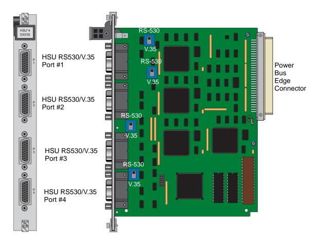
Figure 1-4. Four-Port HSU 530/35 Card Switches
