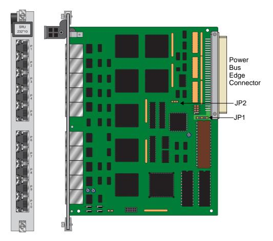
Figure 2-1. SRU 232\*10 Jumper Settings
