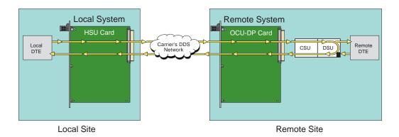
Figure 1-14. Remote DSU Loopback
