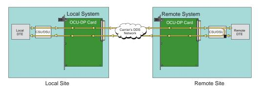
Figure 3-7. OCU Remote Loopback (csu-n option)
