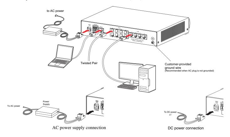
The EtherXtend device provides the loop bonding among all SHDSL ports or a single SHDSL connection. Link-up time can vary depending on the quality, gauge and distance of the copper cables. Model information is displayed on the bottom of the device. When the AC plug is not grounded, ground the device using minimum 16-guage wire tied to a building or earth ground.
