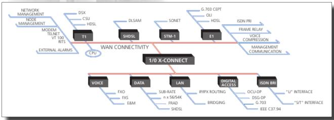
IMACS patented bus architecture simultaneously supports circuit, packet, and cell-switching on a single platform
