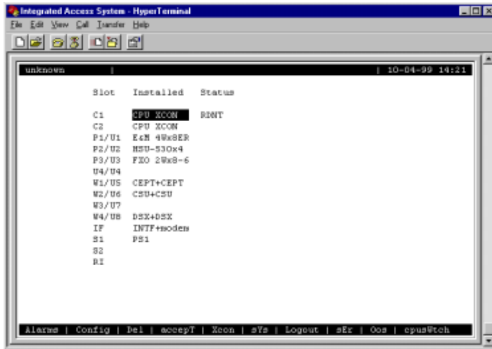
Figure 4-64. Typical System with CPU Switchover Completed
