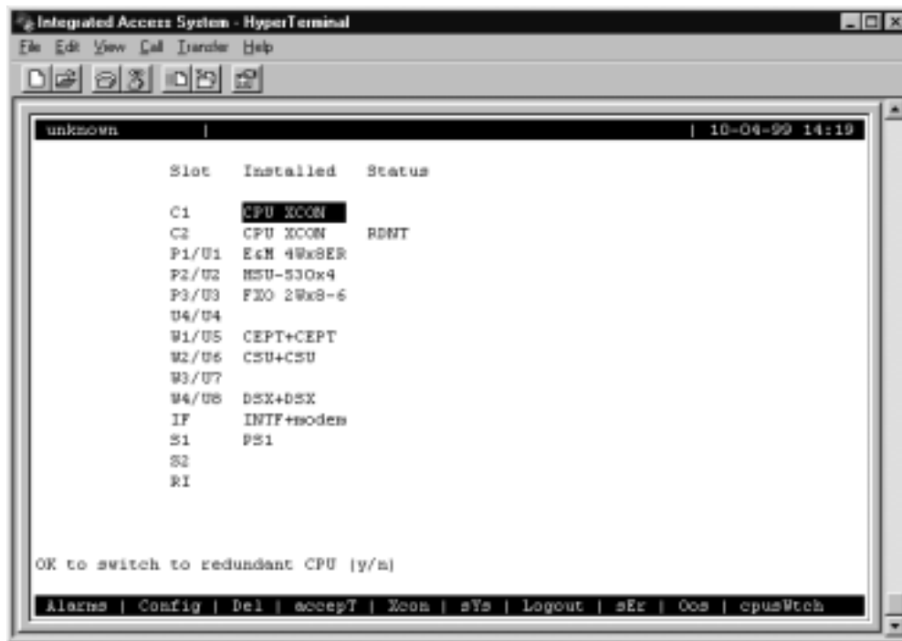
Figure 4-63. Manually Switching to a Redundant CPU
