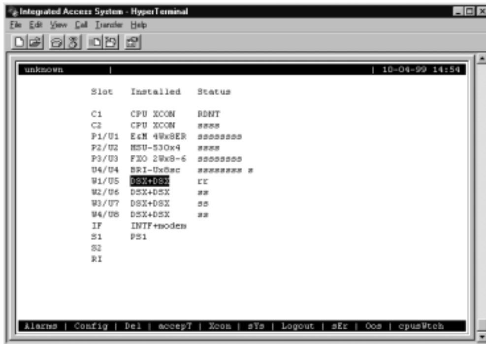
Figure 4-67. Typical Cross-Connect WAN Card Redundancy Switch in Progress
