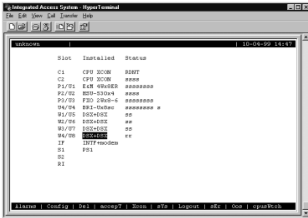
Figure 4-65. Typical Cross-Connect System with WAN Card Redundancy
