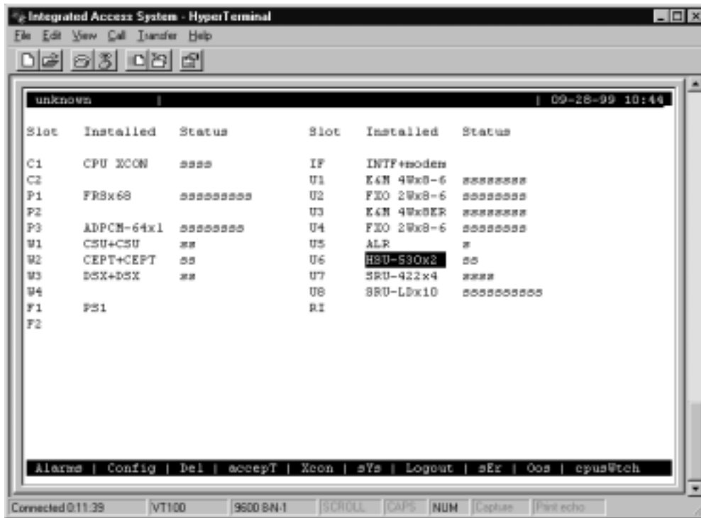
Figure 4-9. Typical Card Status Display
