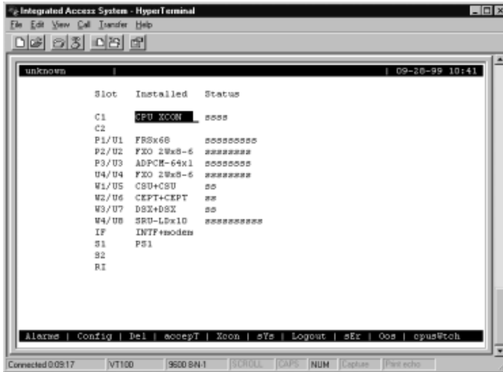
Figure 4-8. Typical System Main Screen (Front-Loading Chassis with Power Supplies on the Side)
