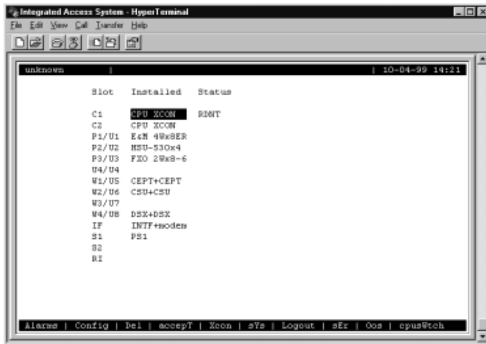
Figure 4-64. Typical System with CPU Switchover Completed
