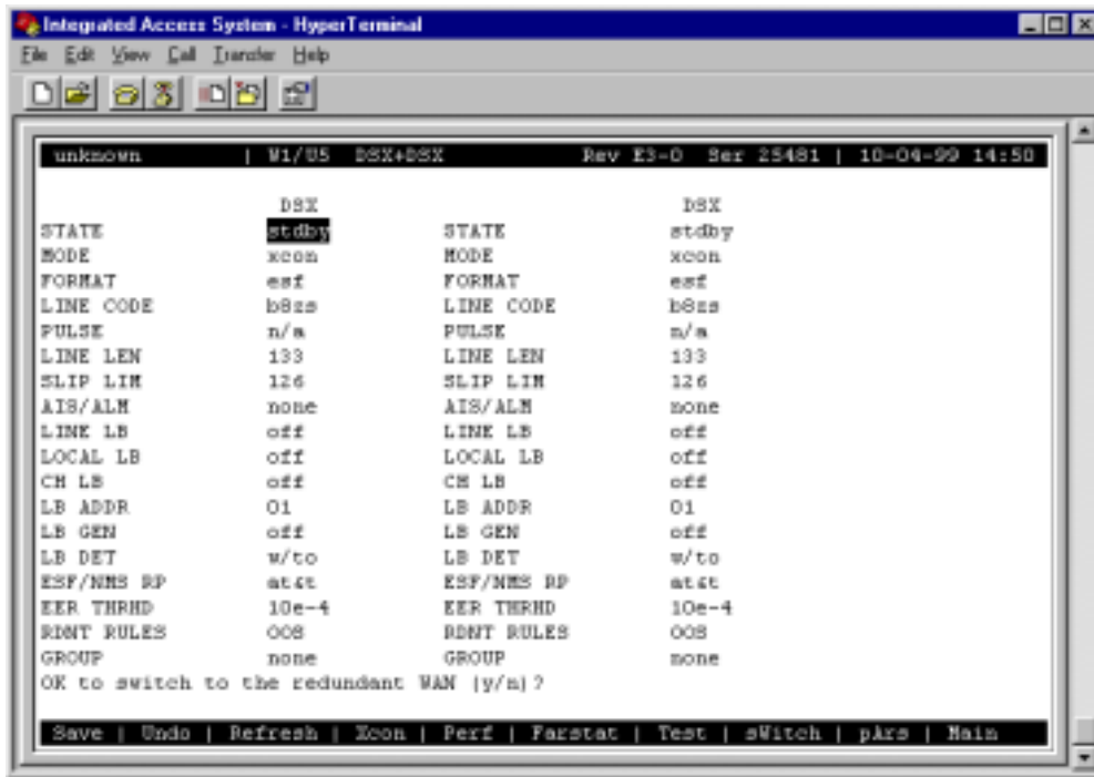
Figure 4-66. Switching to a Redundant Cross-Connect WAN Card
