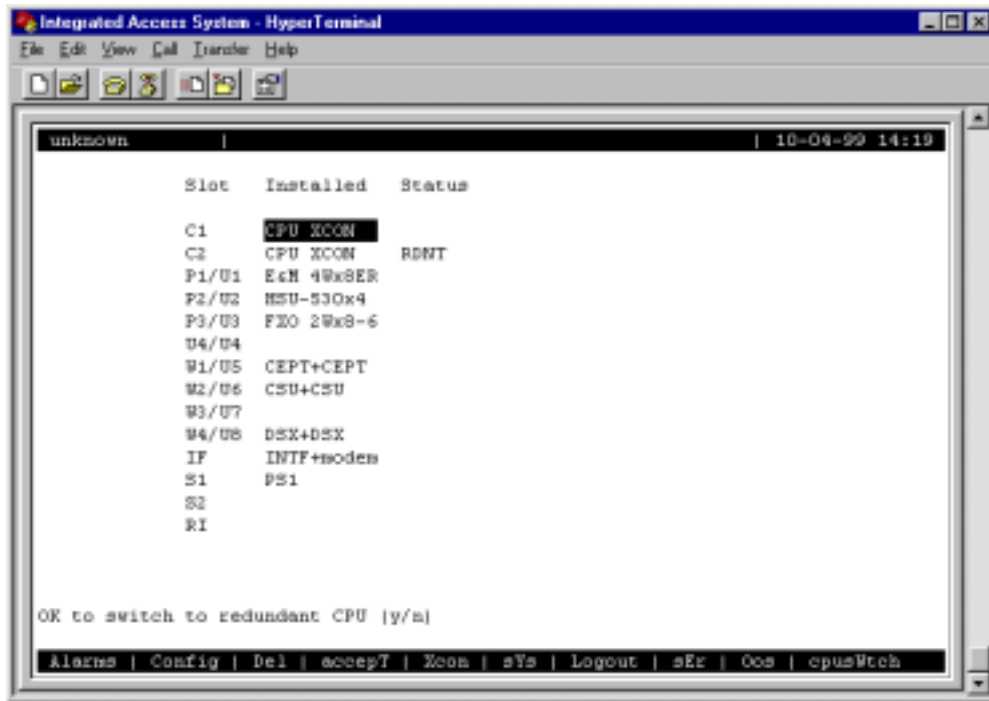
Figure 4-63. Manually Switching to a Redundant CPU
