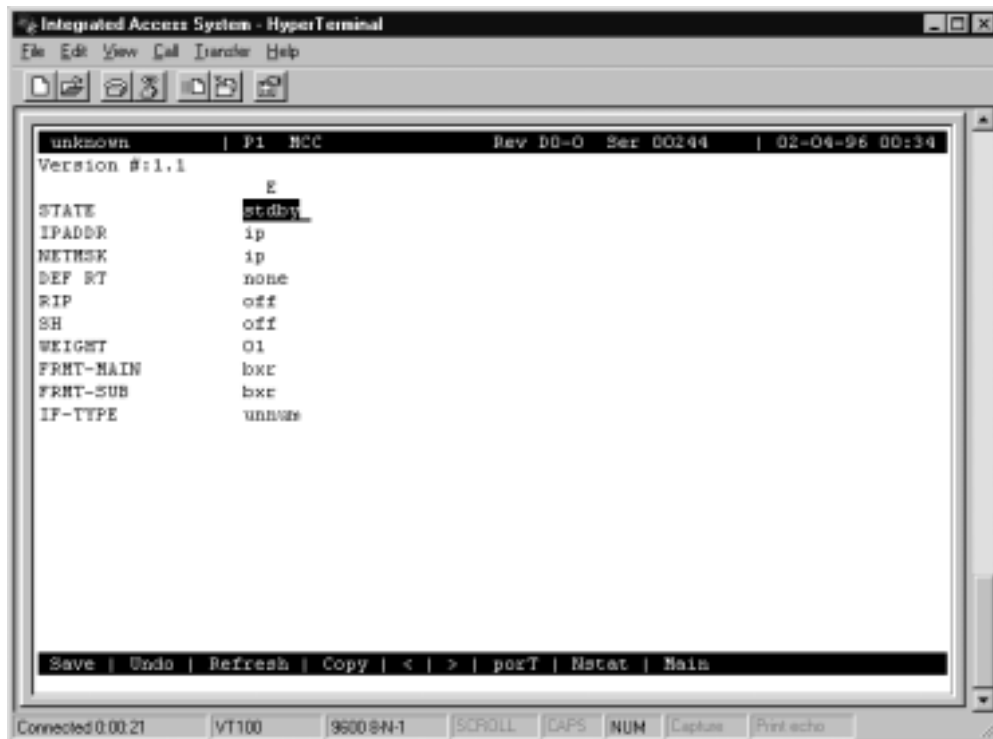
Figure 3-2. Typical ACS-MCC Card Main Screen
