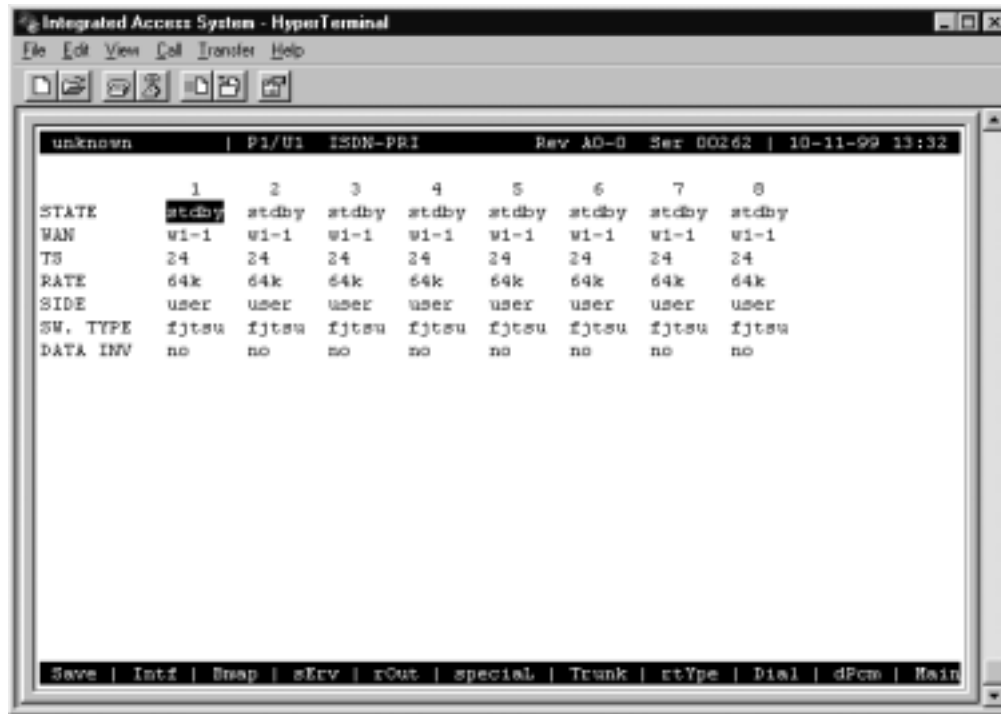
Figure 5-8.D Channel Configuration Screen
