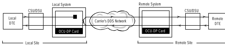
Figure 3-5. OCU Local Loopback (net-d option)
