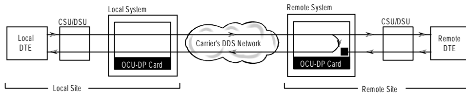
Figure 3-6. OCU Remote Loopback (ds0-n and ocu-n options)
