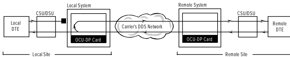
Figure 3-4. OCU Local Loopback (net-a option)
