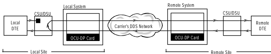
Figure 3-11. OCU Remote Loopback (csu-u option)
