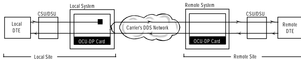
Figure 3-8. OCU Local Loopback (net-d option)
