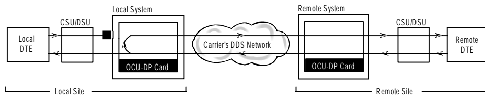
Figure 3-7. OCU Local Loopback (net-a option)
