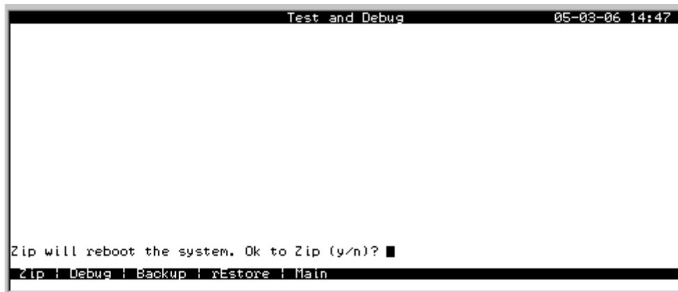
Figure 3-9. Cold-Start NVRAM "Zip" Test and Debug Screen.
