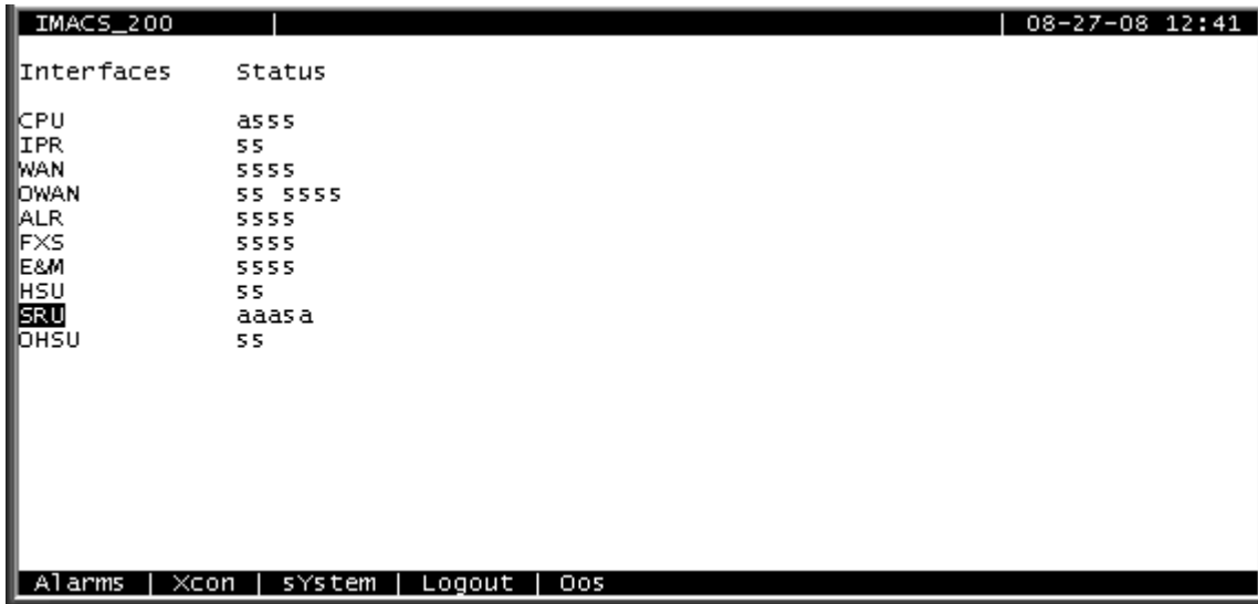
Figure 11-2. Alarm Level from the Main Screen
