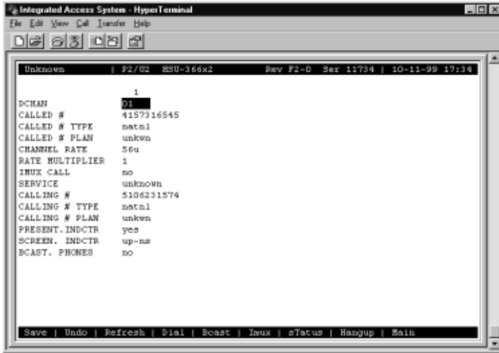
Figure 7-5. HSU Card Call Profile Screen
