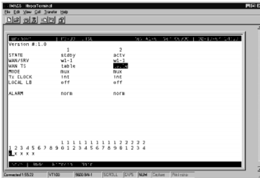
Figure 2-4. Typical OHSU Port Time Slot Assignment Screen
