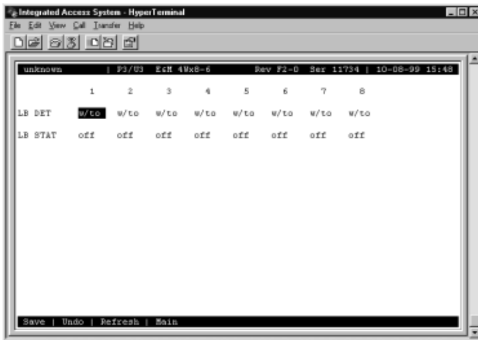
Figure 1-6. Typical E&M Loopback Screen
