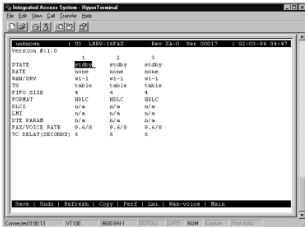
Figure 7-4.LBRV-16 FAX Card Main Configuration Screen
