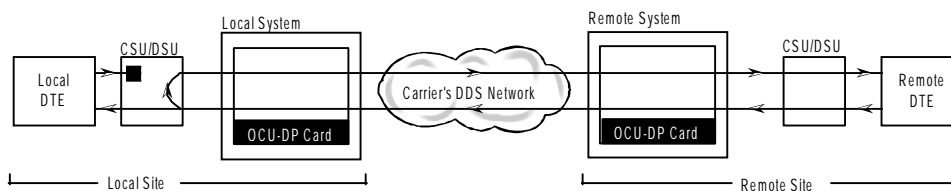
Figure 3-8. OCU Remote Loopback (csu-u option)
