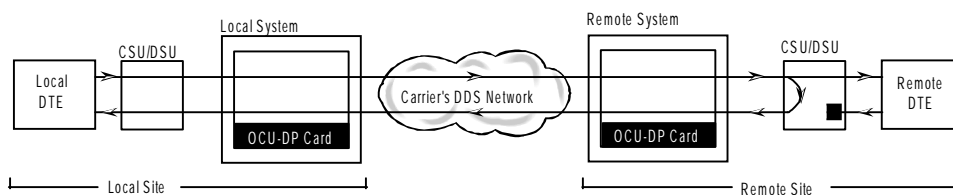
Figure 3-7. OCU Remote Loopback (csu-n option)
