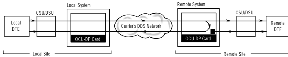
Figure 3-6. OCU Remote Loopback (ds0-n and ocu-n options)
