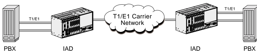
Figure 4-6.IAD using ADPCM for PBX to PBX Application
