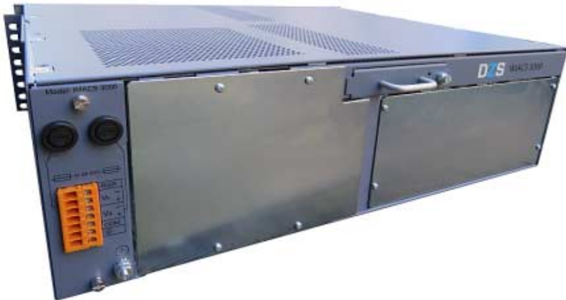
Figure 2-2. Rear of IMACS 3000 with shipping plates
