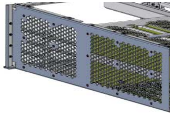
Figure 2-3. Chassis side mounting holes
