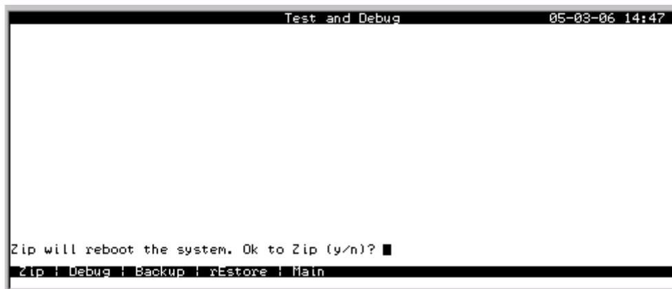
Figure 3-9. Cold-Start NVRAM "Zip" Test and Debug Screen.
