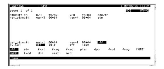
Figure 3-28. Supported Signaling Trunk Conditioning Types
