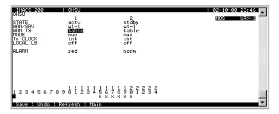
Figure 10-3. Typical OHSU Port Time Slot Assignment Screen
