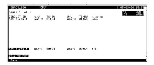
Figure 3-25.New Circuit Selection and ID Assignment
