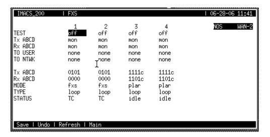
Figure 6-4. Typical FXS port Test Screen
