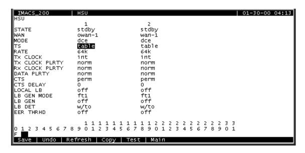
Figure 9-2.HSU Port Time Slot Assignment Screen
