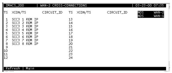
Figure 4-13. Displaying the SCC ports
