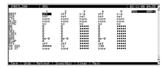
Figure 8-4. Typical SRU port Test Screen
