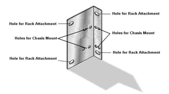
**Figure 2-2. Mounting Bracket Holes**
