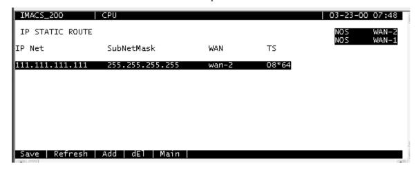
Figure 4-14. Setting up a Static IP Route on the IMACS-200
