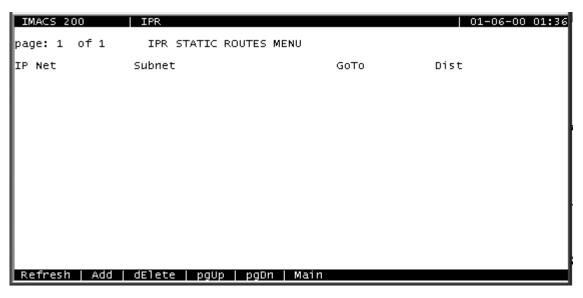
Figure 12-9.IPR IP Static Routes Configuration Menu Screen
