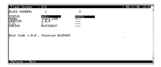
Figure 4-22.Flash Screen with Software Removed
