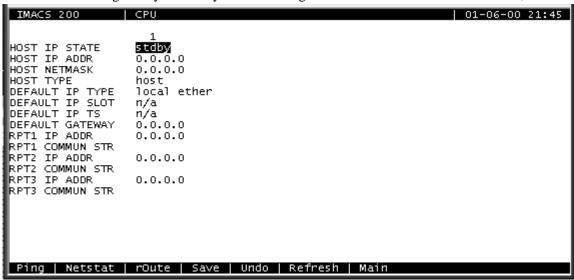
Figure 3-15. Setting the Host IP address
