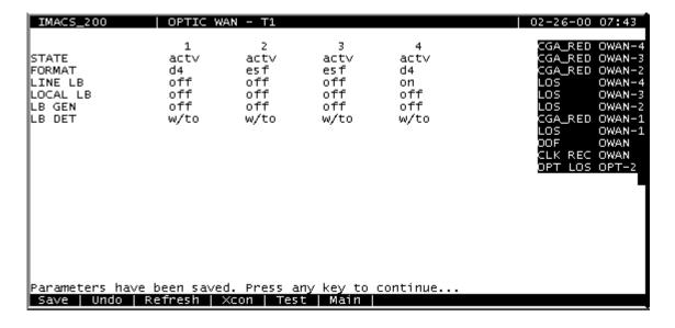
Figure 13-4. Typical Settings for the T1 OWAN Ports
