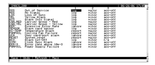
Figure 11-1. Alarm Filter Screen
