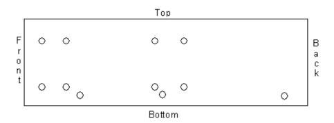
Figure 2-3. Chassis Mounting Holes
