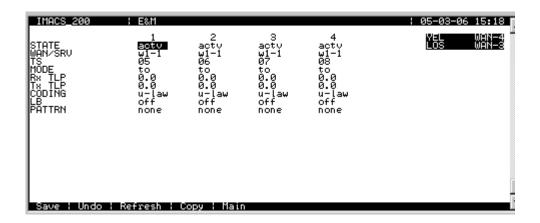
Figure 3-16. Typical E&M port Time Slot Assignments
