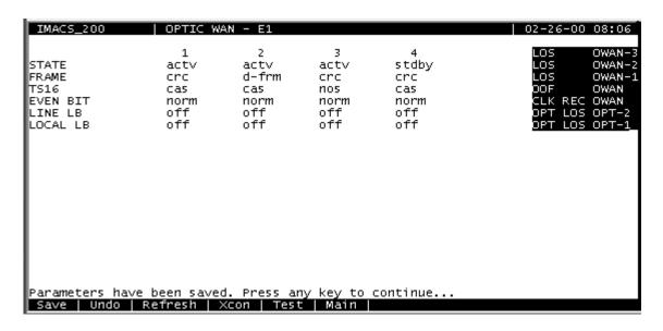
Figure 13-5. Typical Settings for the E1 OWAN Ports
