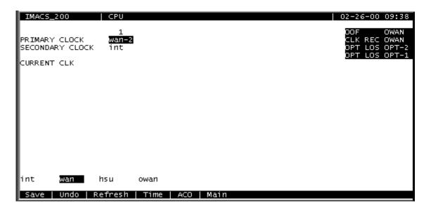
Figure 4-8. Setting the System Clock Source
